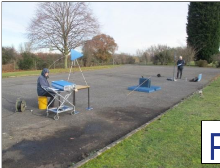
BLU antenna: Bow-tie Low Freq. Ultra-Wideband antenna
