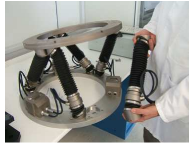
Reduction of the gravitational effects using a hexapod to position the sub-reflector
