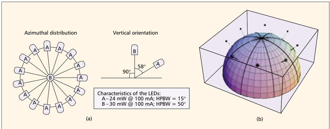
■ Figure 4. a) Distribution and orientation of the infrared LEDs of the optical transmitter; b) optical structure of the angle diversity receiver with eight sectors uniformly distributed.
