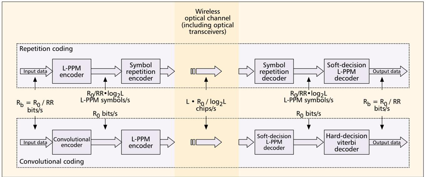
■ **Figure 2.** Block diagrams of L-PPM adaptive data rate systems with soft-decision L-PPM decoding employing repetition coding and convolutional coding with a hard decision Viterbi decoder.
