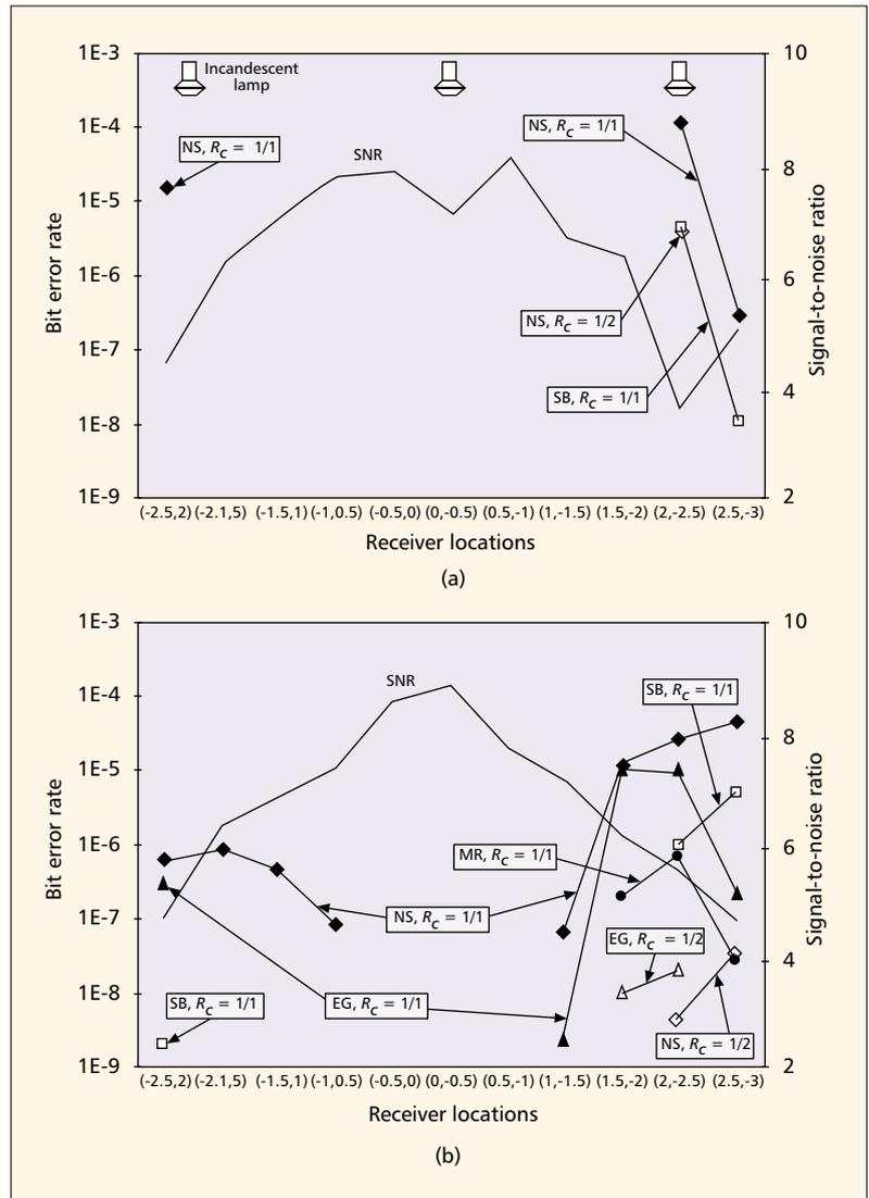
■ Figure 5. Bit error rate measured over the diagonal line considering a) incandescent and b) fluorescent illumination.
