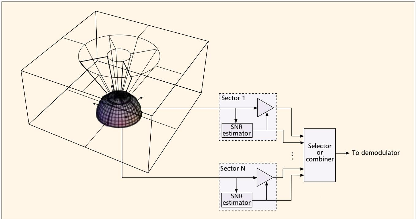
■ **Figure 3.** The general structure of an angle diversity receiver.
