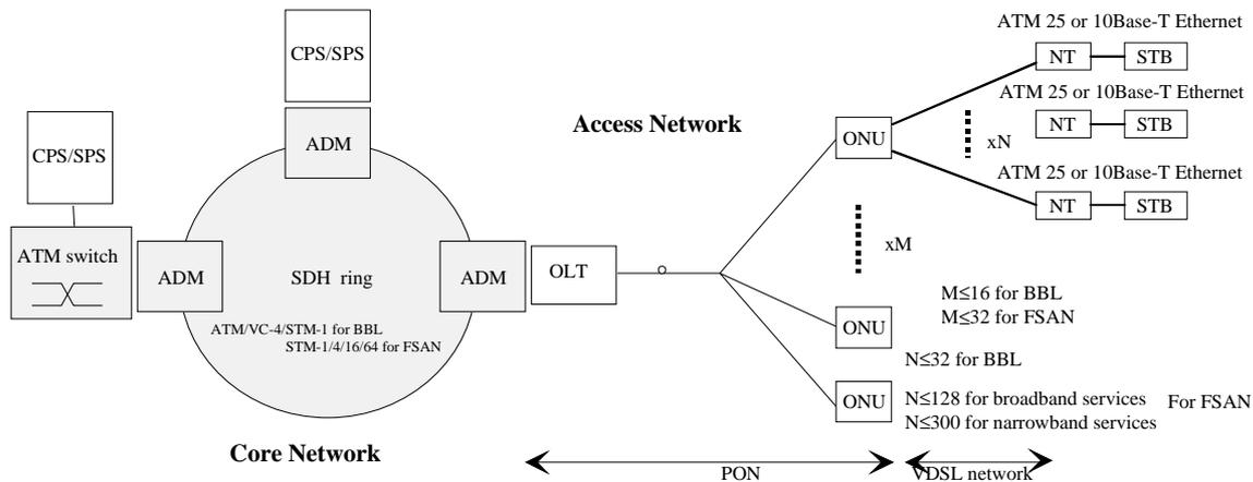
Figure 1. BroadbandLoop system architecture.
