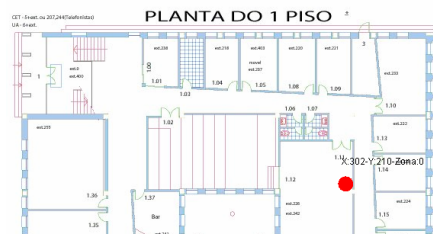
Fig. 2. Wireless client position using a floor plan
