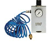
ZelFlex frames must be refilled with compressed air for 5-10 s to provide the necessary stretching force.
