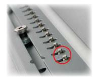
Stencil supporting pins on the stretching bar enable a fast and easy placement of stencils onto the ZelFlex frame.
