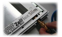
Release air from the ZelFlex frame: use the air connector (connection hose) → push the female thread towards the male thread just enough to release the clamp (do not connect)
