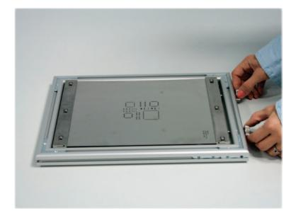
The gap between the locker on the stretching screw and the bar should be approx. 3 mm for the required working tension.
