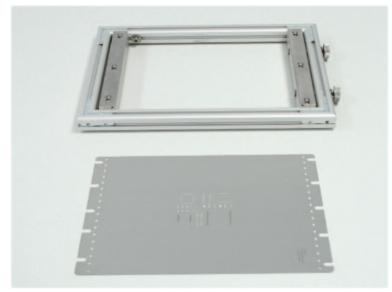
Using the two hexagon-headed screws, attach the rear bar according to the stencil length. Tighten them (the rear bar must be parallel to the rear frame profile).
