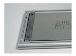
8. Place the stencil onto the pins on the front stretching bar.
