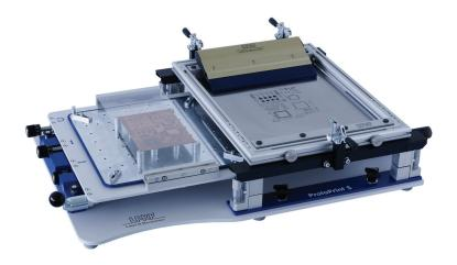
The printer should only be used in a dry environment, on a suitable flat surface, e.g. a work table. There must be a free area of at least 1000 × 900 mm around the machine to allow sufficient space for opening the machine and on either side for both non-printed and printed materials.
