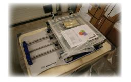
Finally remove the remaining plastic foil around the frame and handle and take out the items enclosed with the printer (User Manual, packing list, accessories etc.).
