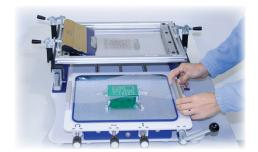
Remove the test print screen from the printing table.
