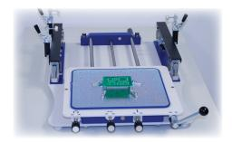
Lay the PCB to the centre of the printing table. Clamp it:
