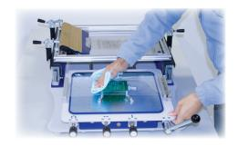
Clean the test print screen with soft a cloth, moistened in isopropyl alcohol.
