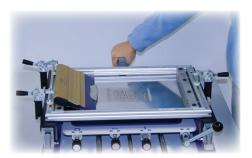
Separate the PCB and test screen from the framed stencil, using the elevating/release lever.
