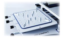
Clamping of a PCB can be easily done with the provided supporting pins.
