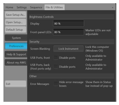
**Brightness controls.** Adjust the brightness levels of the display and front panel LEDs.
