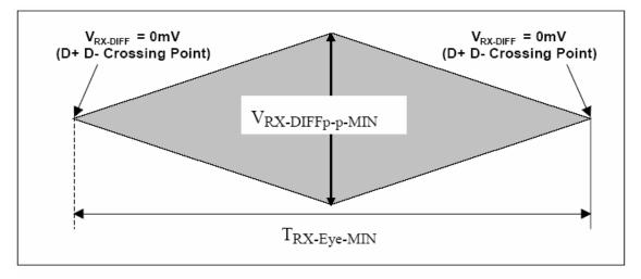
Figure 2: Receiver input eye voltage and timing specifications
