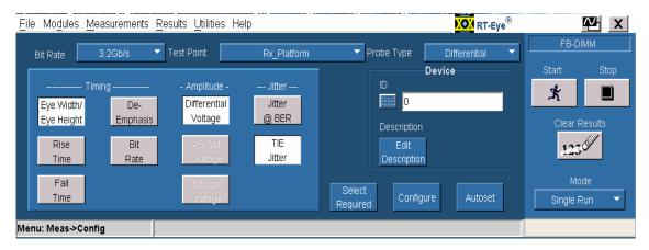
Figure 6b: Measurements select menu setup for Receiver Platform test point with SSC off when tested using the TDSN4238B/Intel's DLB fixture
