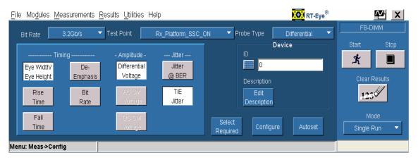
Figure 6c: Measurements select menu setup for Receiver Platform test point with SSC on when tested using the TDSN4238B/Intel's DLB fixture
