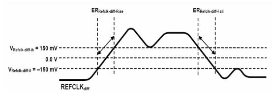
Figure 15: Reference clock rise/fall time calculation
