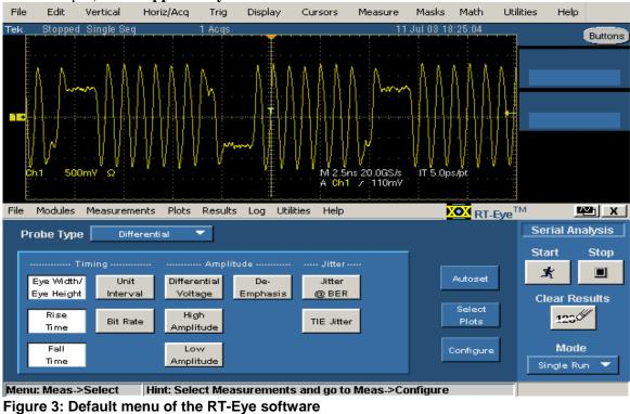
Figure 3 shows the oscilloscope display. The default mode of the software is the **Serial Analysis** module (Opt. RTE-Version 2.0). This software is intended for generalized Serial Data analysis on 8B/10B encoded copper links.
