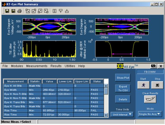
Figure 10 shows the result of a Transmitter Compliance test on a signal that passes the transmitter tests at TX compliance test points.
