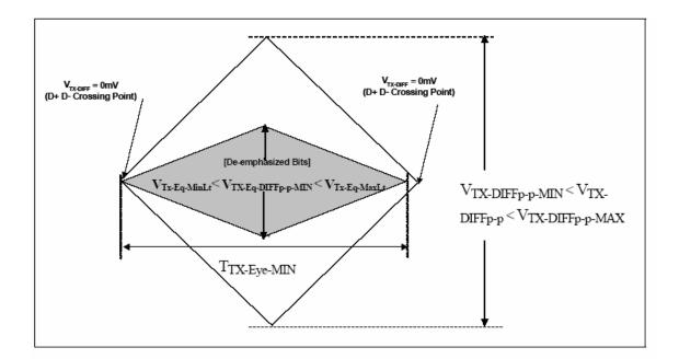
Figure 1: Transmitter output eye specifications, with and without de-emphasis
