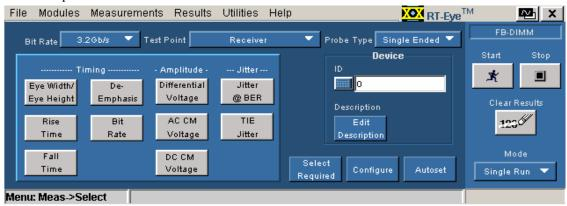
Figure 6a: Measurements select menu setup for Receiver test point as per FBDIMM spec
