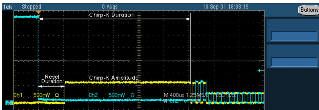
The TDSUSB2 application automates this process and automatically generates the [results \(see page 86\)](#) and reports for the results of Chirp-K duration, Chirp-K amplitude, and Reset duration.
