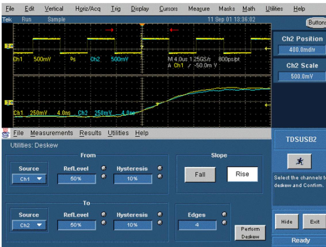
19. The zoomed section of the waveform available on the lower part of the screen shows the results of the deskew operation clearly. You will see that after performing the deskew operation, the skew is automatically removed.
