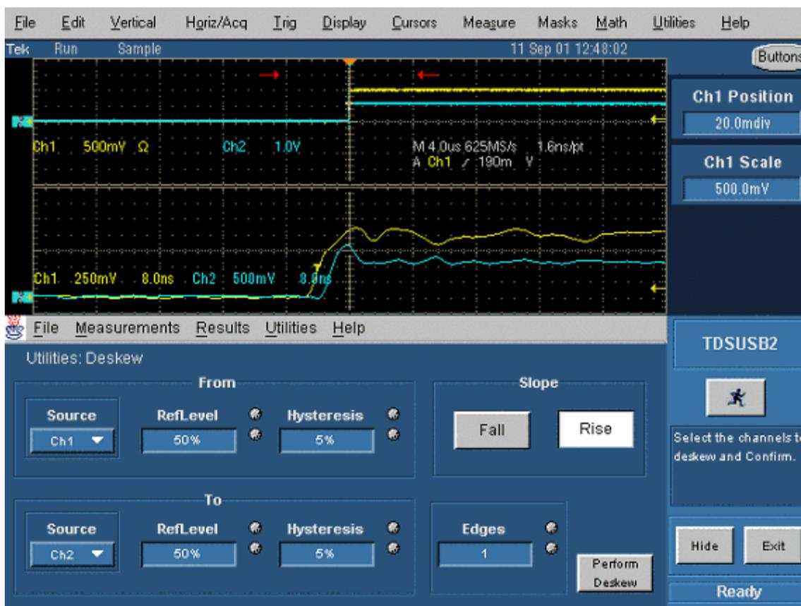
4. To start the application from a supported oscilloscope, select File > Run Application > USB2.0 Test Package from the menu bar of the oscilloscope.
