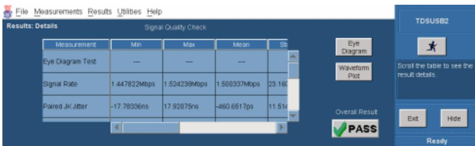
**NOTE.** The application displays the user column in the Results Details only if the User Configurable Limits are selected in File > Preferences > Advanced tab.
