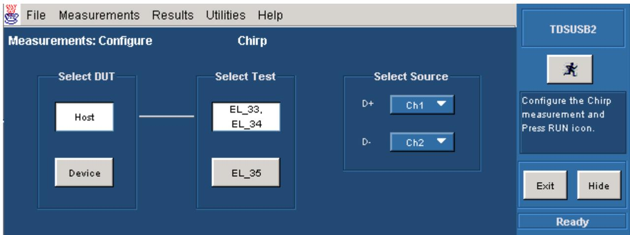
4. Select the Host option to display the different tests for the DUT. The available tests are:
