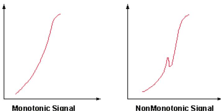
To verify the monotonic behavior of a signal, the oscilloscope must have a sample rate high enough to capture as many sample points as possible on a rising or falling edge. In addition, the oscilloscope should have enough bandwidth to ensure that the high frequency non-monotonic transition is not attenuated.
