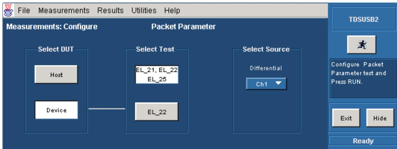
5. Select the Device option to display the different tests for the DUT. The available tests are:
