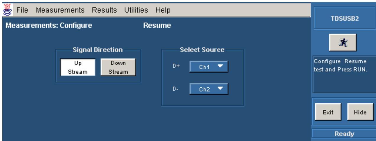
3. Set the input Signal Direction to either Upstream or Downstream.
