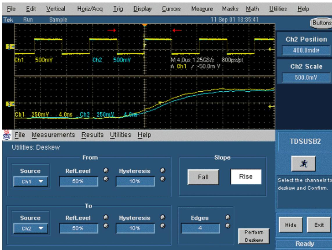
18. Set the Reference levels for Ch1 and Ch2 in the application to 50%, the hysteresis to 10%, the number of edges to 4, and the type to rising edge.
