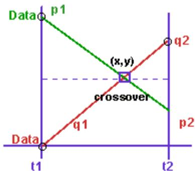
The intersection of the four voltage points p1, p2, q1, and q2 gives the Cross-Over point for Voltage level (y) and time (x). x and y coordinates are obtained by solving the following two equations:
