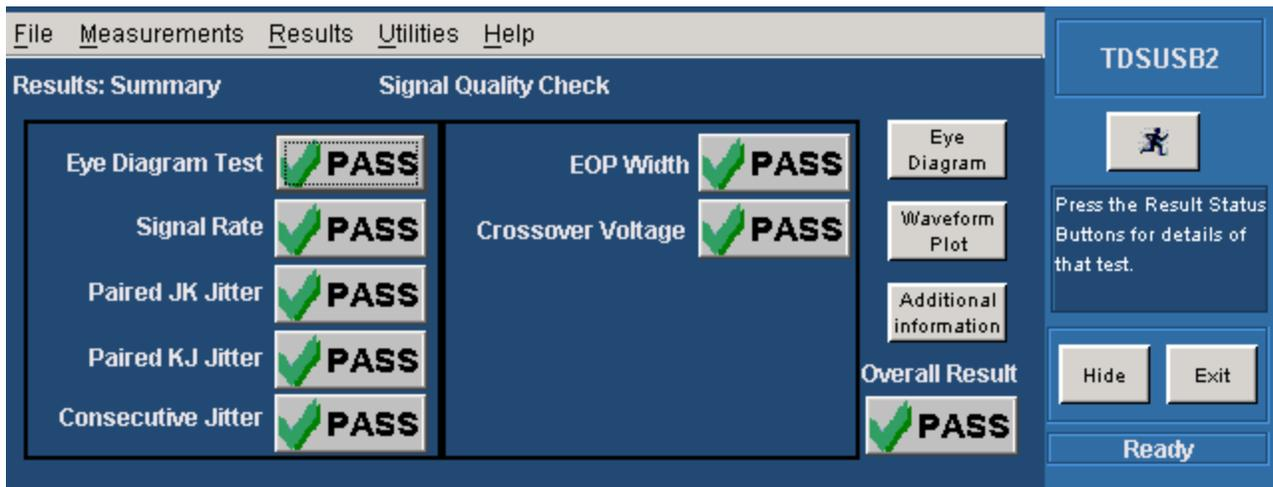
2. Click on any of the test result buttons to get the details of that test.
