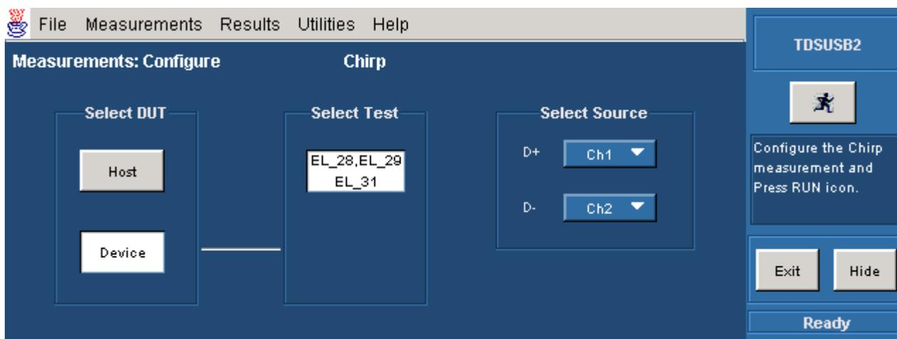
5. Select the Device option to display the different tests for the DUT. The available tests are:
