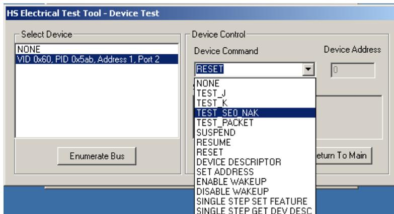
Figure 29: Device TEST\_SE0\_NAK
