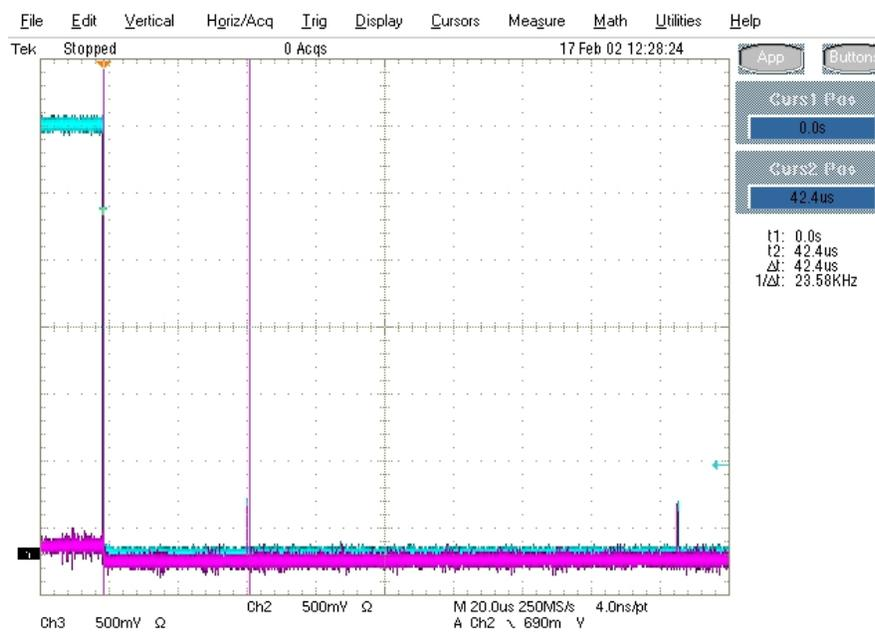
Figure 22: Device Resume to High-speed
