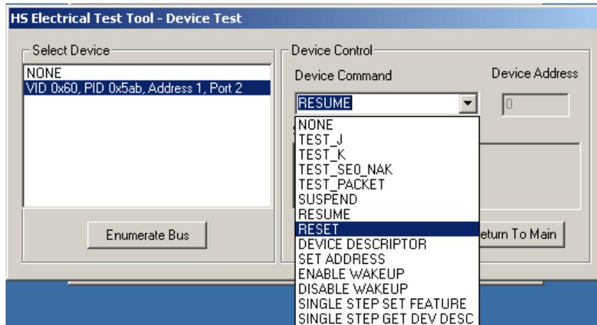
Figure 26: Device Reset
