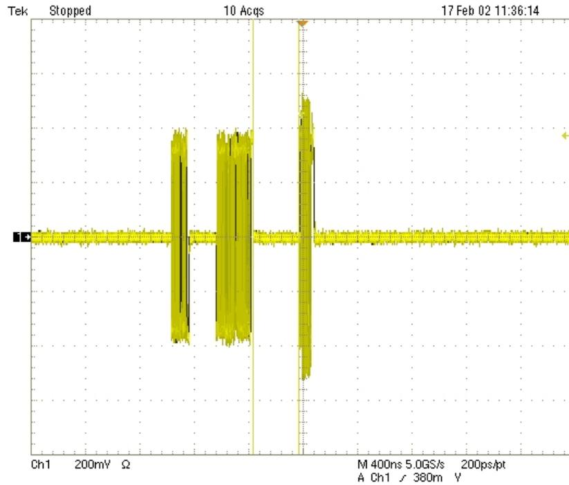
Figure 14: Device Inter-packet Gap
