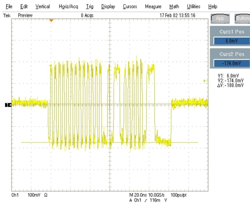
Figure 32: Measuring Differential Voltage Level – Zero to Negative Peak
