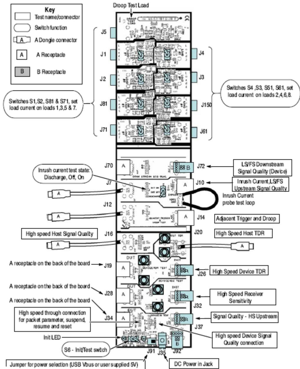
Figure 1: Tektronix TDSUSBF Test Fixture
