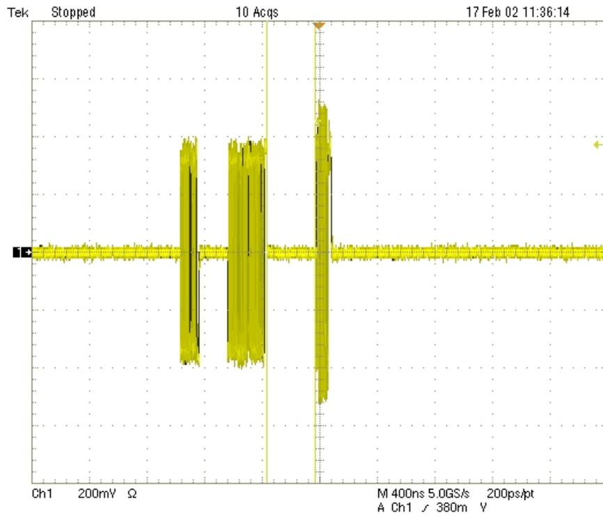
Figure 11: Host and Device Packets
