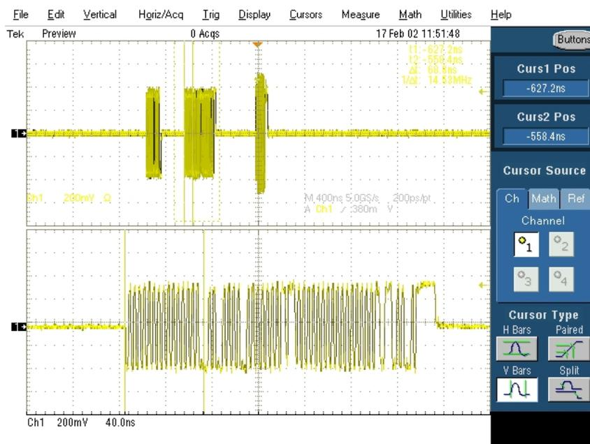
Figure 12: Sync Field – Device Packet
