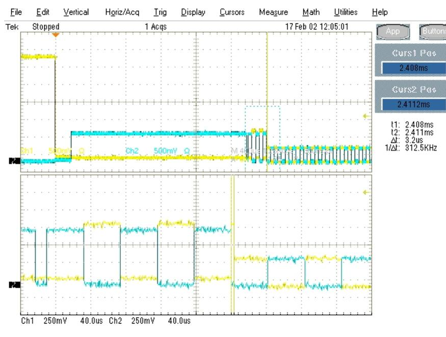
Figure 18: Time From Start of Last J in Chirp K-J-K-J-K-J To Device Turns on HS Termination
