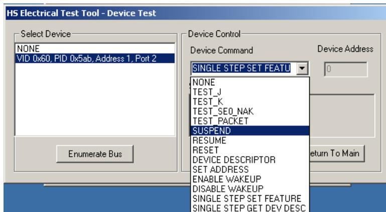
Figure 25: Device Suspend
