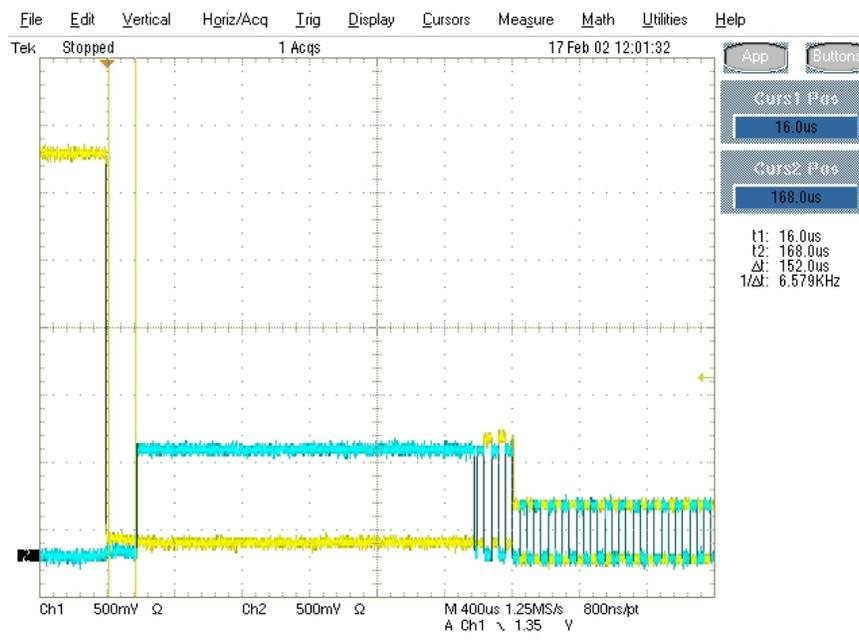
Figure 17: Device Chirp-K Latency
