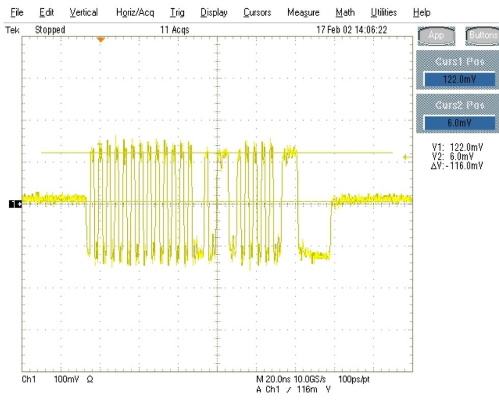
Figure 33: Measuring Differential Voltage Level – Zero to Positive Peak
