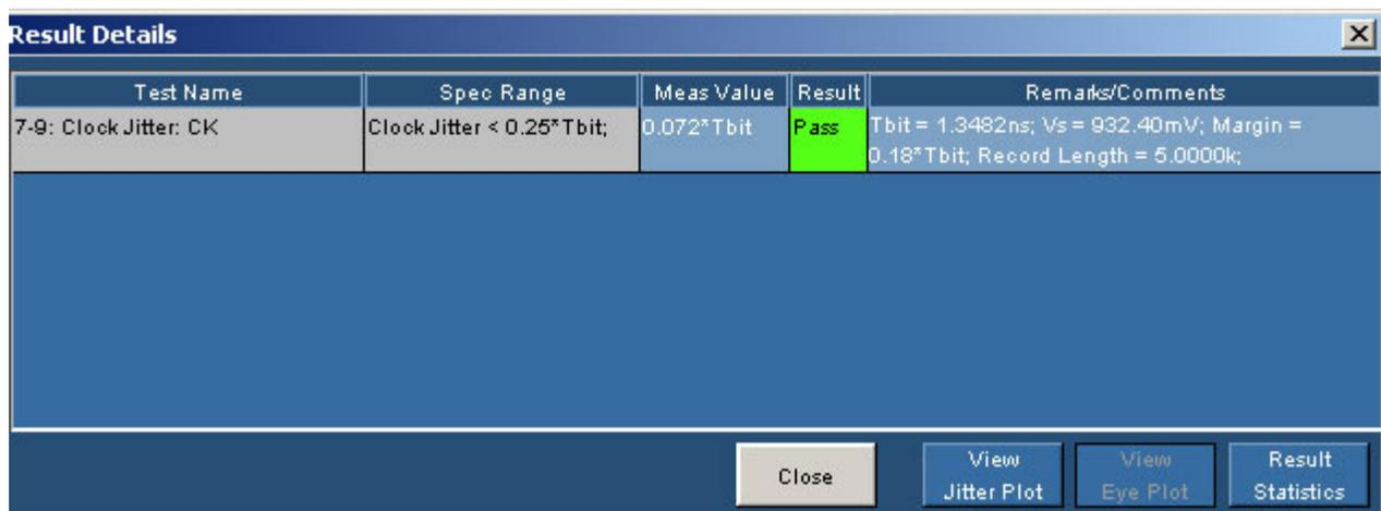
Figure 133: Result Details for Clock Jitter
