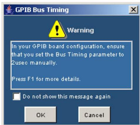
**Figure 35: GPIB Bus Timing dialog box**
