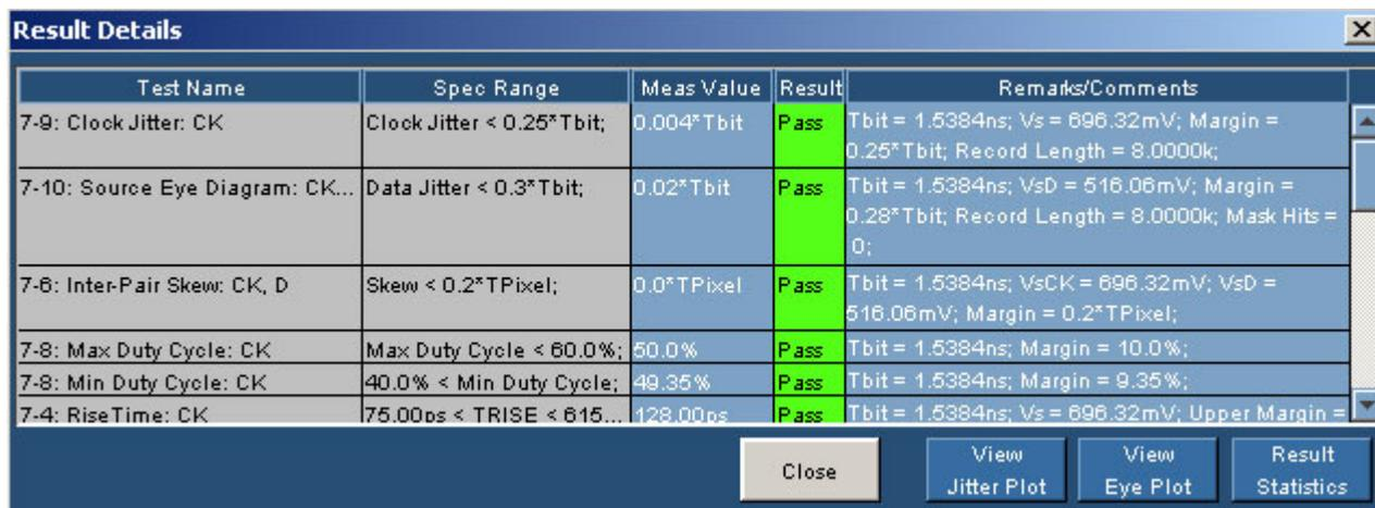
Figure 162: Result Details for Source Multiple Tests
