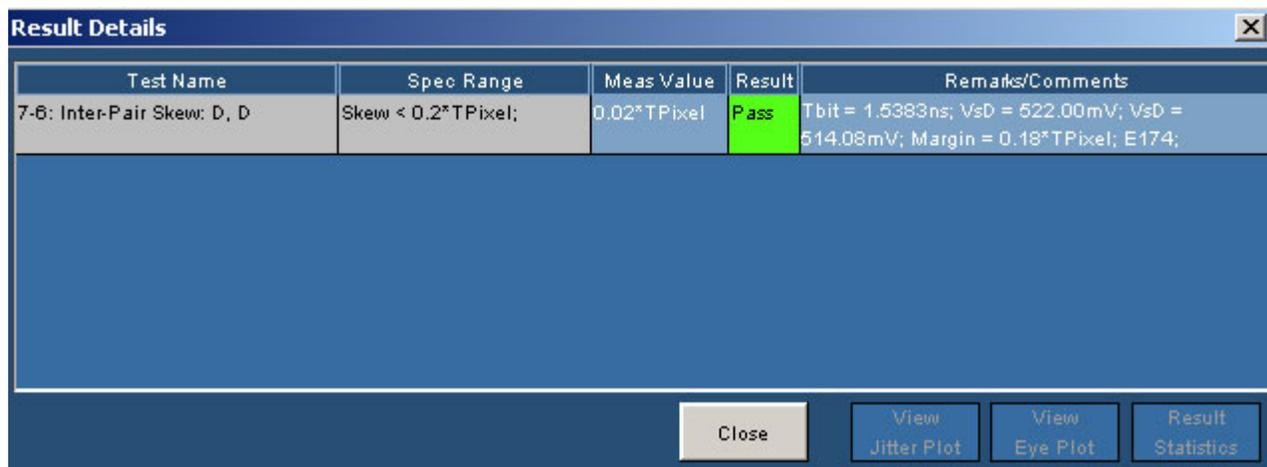
Figure 170: Result Details for Inter-Pair Skew (Data-Data)
