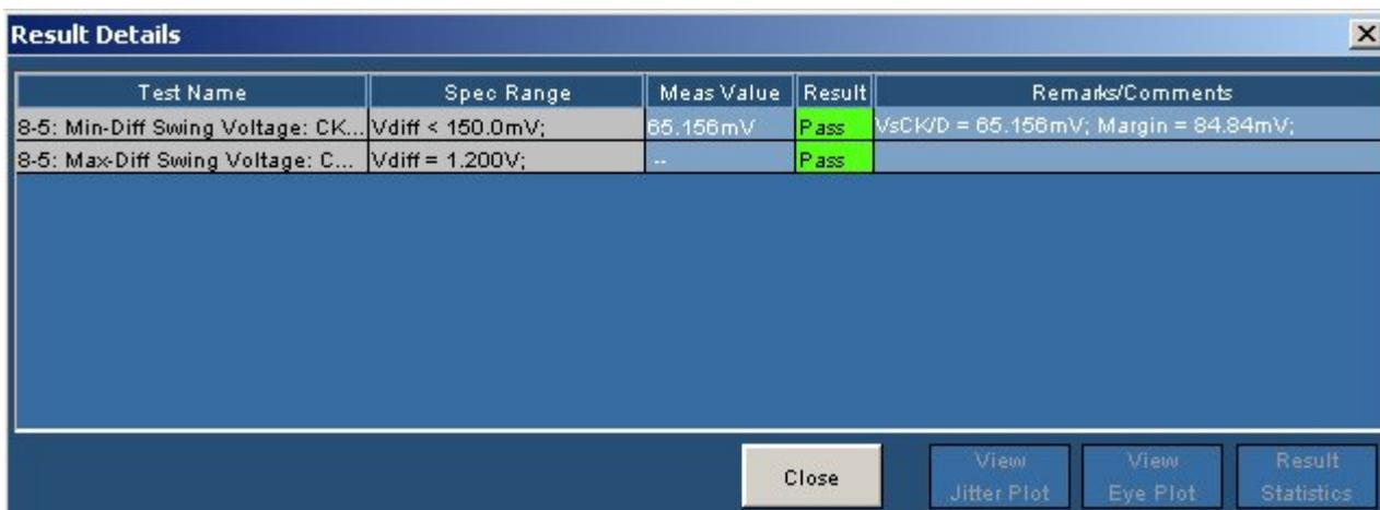
Figure 198: Result Details for Min/Max-Diff Swing Tolerance
