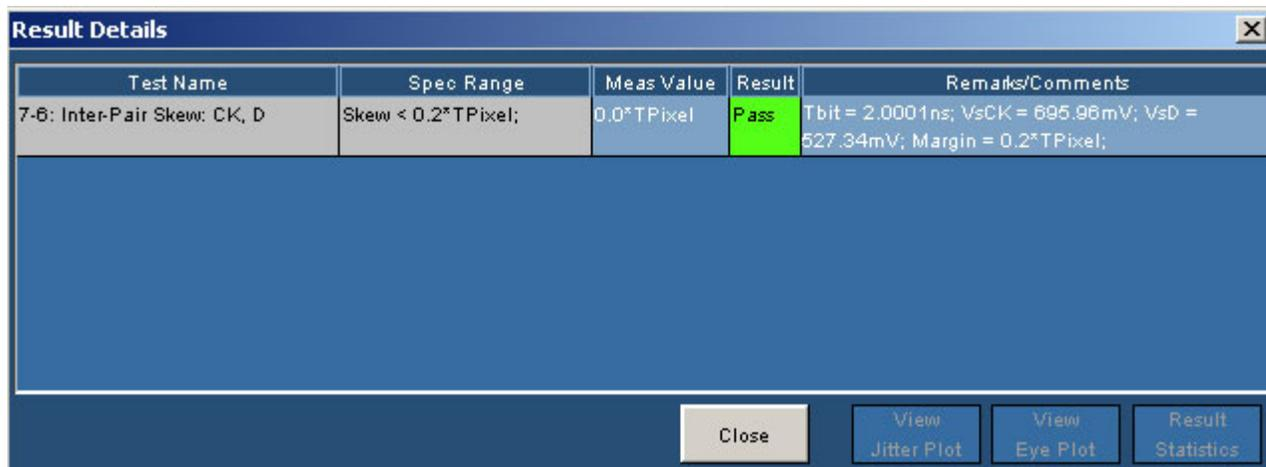
Figure 155: Result Details for Inter-pair Skew (Clock-Data)
