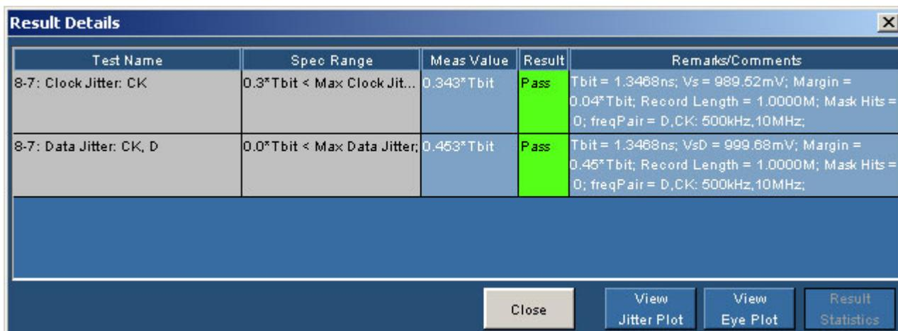
**Figure 208: Result Details for Jitter Tolerance**
