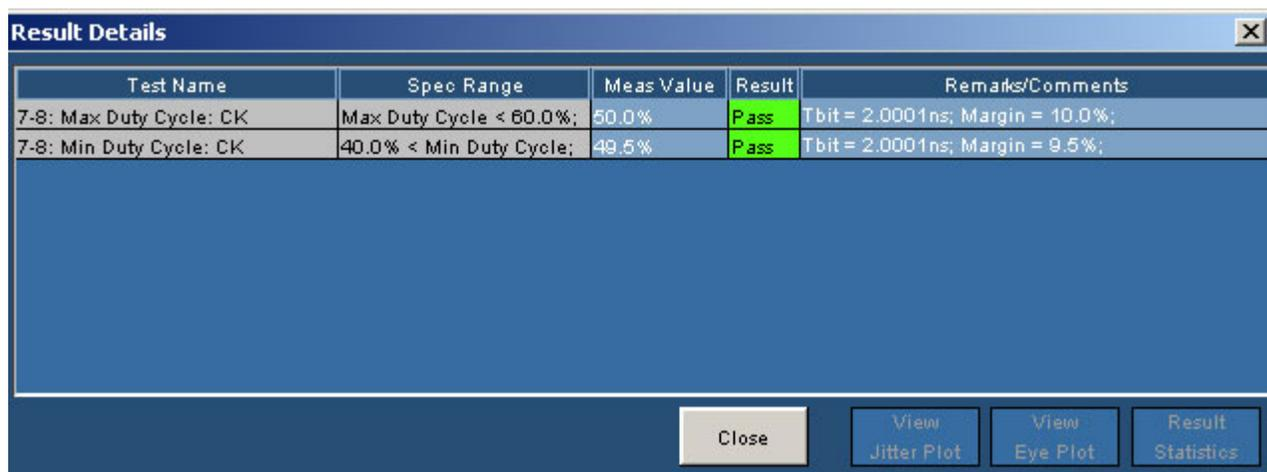
Figure 110: Result Details for Duty Cycle
