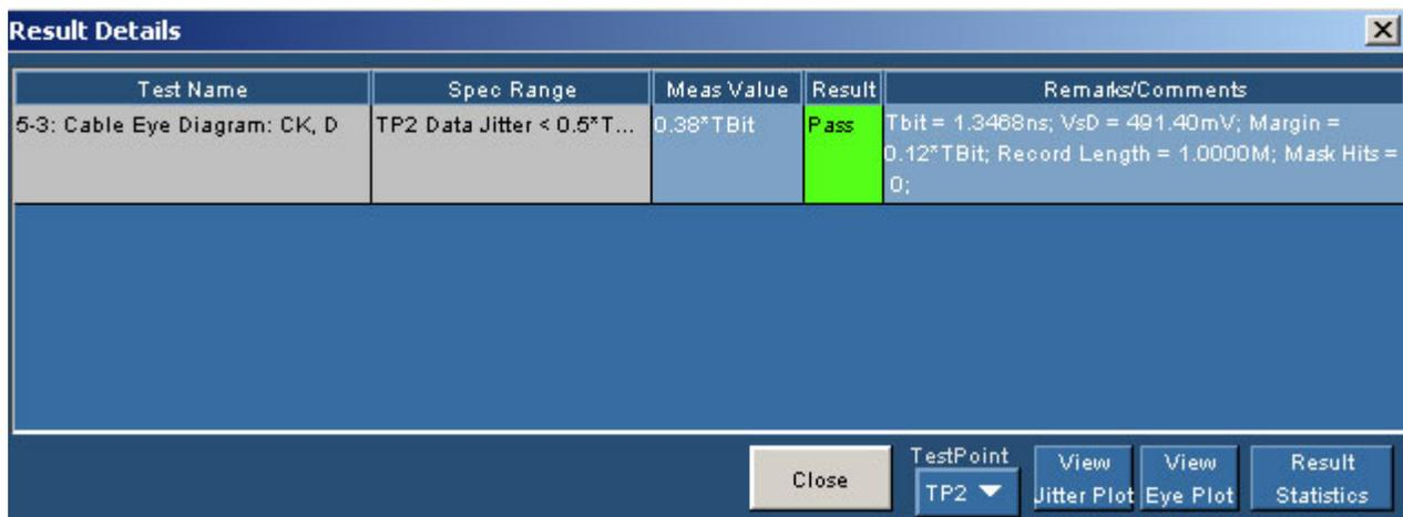
Figure 223: Result Details for Cable Eye Diagram
