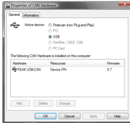
Figure 8: Dialog box for selection of the used CAN hardware (here: PCAN-USB interface)
