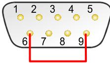
Figure 6: Schematic representation of a connection between the pins "+U<sub>b1</sub>" (6) and "Boot CAN1" (9) on the CAN 1 D-Sub connector (IPEH-002210 only)
