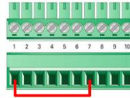
Figure 7: Schematic representation of a connection between the pins "+U<sub>b</sub>" (1) and "Boot CAN1" (7) on the screw terminal block (IPEH-002210-P only)
