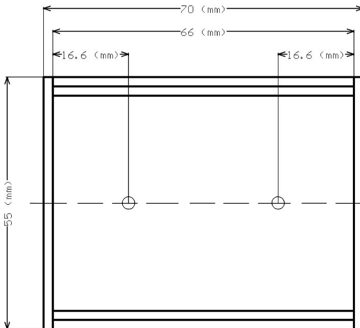
Figure 15: Plan view of the PCAN-Router housing
