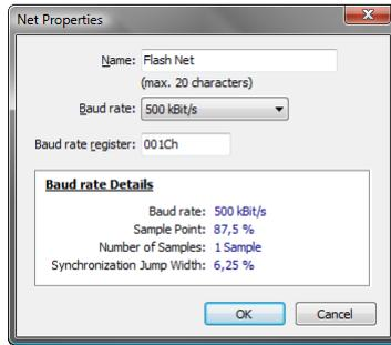
Figure 10: Setting up a new net with a transfer rate of 500 kBit/s
