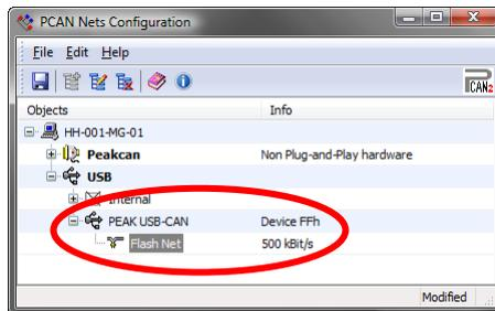
Figure 9: A PCAN net with 500 kBit/s is assigned to the PCAN-USB interface.
