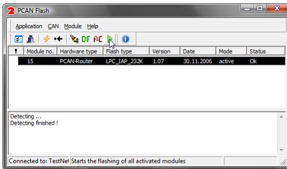
Figure 13: Firmware upload start
