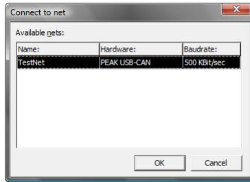
Figure 12: Selection of the CAN network connected to the PCAN-USB interface
