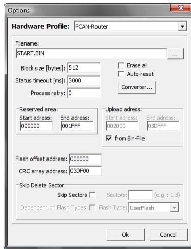
Figure 11: The **Options** dialog box with a selected firmware file
