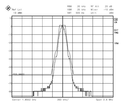
Fig 5 Spectrum due to modulation at fc  $\pm$  1.8 MHz measured with the rms detector
