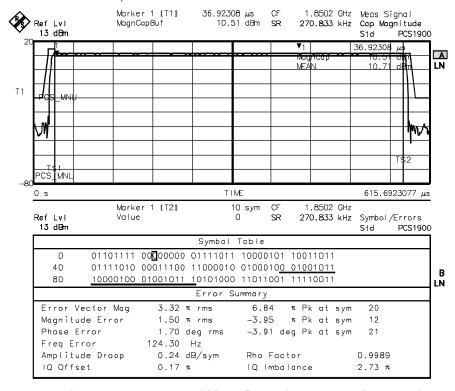
Fig 2 Display for power vs. time measurement and Mean Power in vector analyzer mode
