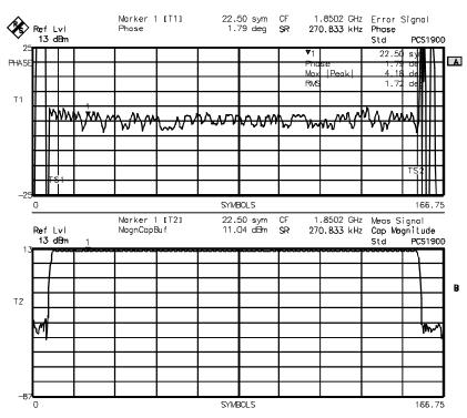
Fig 1 Display of PCS1900 phase error measurement
