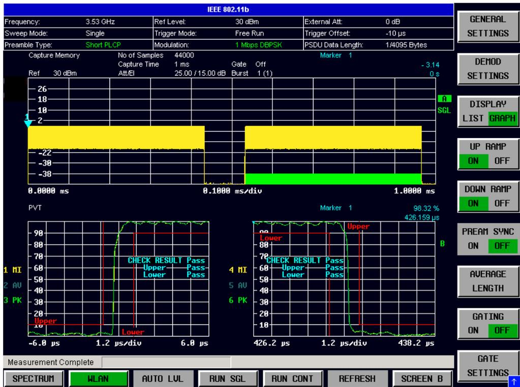
Fig. 2-7 PVT Results – Up Ramp and Down Ramp Switched On
