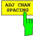
The *ADJ CHAN SPACING* softkey opens a table for defining the channel spacings.
