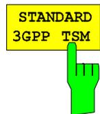
The *STANDARD softkey* selects, whether the measurements are based on the 3GPP standard or the TSM standard. At the moment, this affects the spectrum emission mask measurement only.
