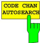
The *CODE CHAN AUTOSEARCH* softkey supports measurements of the code domain power analyzer in automatic search mode. This mode searches the whole code domain (all permissible symbol rates and channel numbers) for active channels. A channel is active when the minimum power you enter, referred to the total power, is exceeded (see *INACT CHAN THRESHOLD* softkey) and there is adequate signal/noise ratio.
