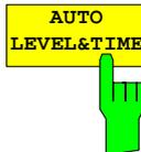
The *AUTO LEVEL & TIME* softkey starts the autorange routine for the reference level. This also creates the relationship between trigger and subframe start.
