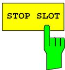
The *STOP SLOT* softkey allows entry of the stop slot for gated sweep mode. The gated mode is on between START SLOT and STOP SLOT. For the remaining slots of a subframe the gated mode is off.
