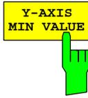
The *Y-AXIS MIN VALUE* softkey sets the lower limit of the displayed probability range. Since the Y-axis scaling is logarithmic, the spacing between the maximum and minimum values must be at least one decade. Permissible range  $0 < \text{value} < 1$ .
