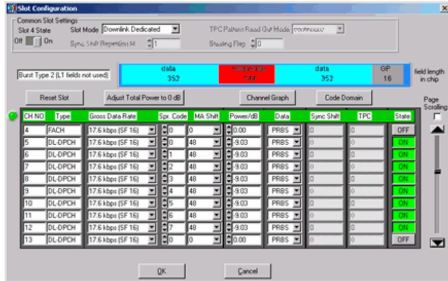
Fig. 2-5 R&S WinIQSIM – channel settings in slots 4-6
