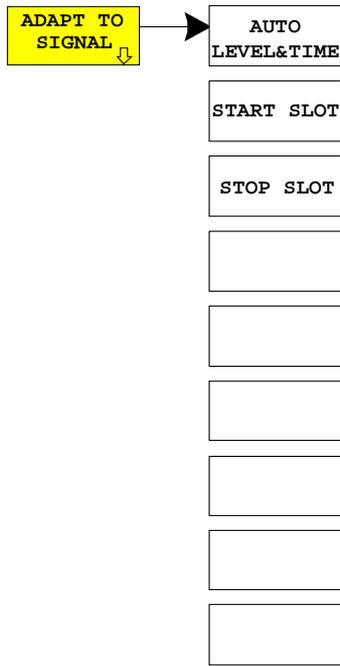
The *ADAPT TO SIGNAL* softkey opens a submenu for matching the reference level of the analyzer and configuration of the gated sweep mode.
