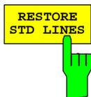
The *RESTORE STD LINES* softkey restores the limit lines defined in the standard to what they were when the unit was supplied. In this way accidental overwriting of the standard lines can be undone.
