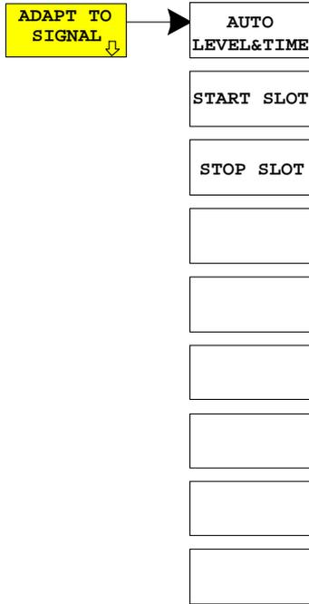
The *ADAPT TO SIGNAL* softkey opens a submenu for matching the reference level of the analyzer and configuration of gated sweep mode.
