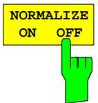
The *NORMALIZE ON / OFF* softkey eliminates the DC offset from the signal. The default setting is *OFF*.
