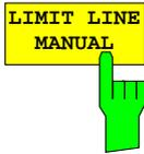
The *LIMIT LINE MANUAL* softkey enables you to select the limit line manually. If you press this softkey, the channel power measurement is not used to select the limit line but only to determine its relative components. The power at the different frequency offsets is compared with the limit line you have specified.
