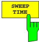
The *SWEEP TIME* softkey activates entry of the sweep time. When the RMS detector is used, a longer sweep time yields more stable results. This setting is identical to the *SWEEP TIME MANUAL* setting in the *BW* menu.
