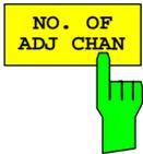
The *NO. OF ADJ CHAN* softkey activates entry of the number  $\pm n$  of adjacent channels that are taken into account for the adjacent channel power measurement.
