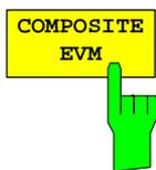
The *COMPOSITE EVM* softkey selects evaluation of error vector magnitude (EVM) over the total signal (modulation accuracy).
