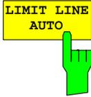
The *LIMIT LINE AUTO* softkey automatically selects the limit line after the power in the useful channel has been determined. If the measurement is performed in a *CONTINUOUS SWEEP* and the channel power varies from sweep to sweep, this can result in continuous replotting of the limit line.
