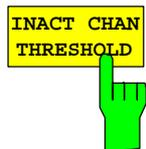
The *INACT CHAN THRESHOLD softkey* allows entry of the minimum relative power that a single channel must have compared to the total signal in order to be regarded as an active channel. Channels below the specified threshold are regarded as inactive.
