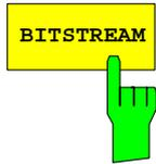
The *BIT STREAM* softkey selects evaluation of the bit stream from the demodulated received signal.
