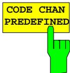
The *CODE CHAN PREDEFINED* softkey switches CDP analysis to the measuring mode with the help of predefined channel tables. In this mode there is no search for active channels in the code domain for the selected slot, instead the channels of a table defined prior to a measurement are assumed to be active.
