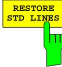
The *RESTORE STD LINES* softkey restores the limit lines defined in the standard to what they were when the unit was supplied. In this way accidental overwriting of the standard lines can be undone.
