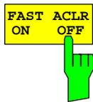
The *FAST ACLR ON / OFF* softkey toggles between measurement by the IBW method (*FAST ACLR OFF*) and measurement in the time domain (*FAST ACLR ON*).
