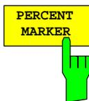
When the CCDF function is enabled, the *PERCENT MARKER* softkey supports positioning of marker 1 by entering a sought probability. In this way the power which exceeds a specified probability can be determined in a simple manner.
