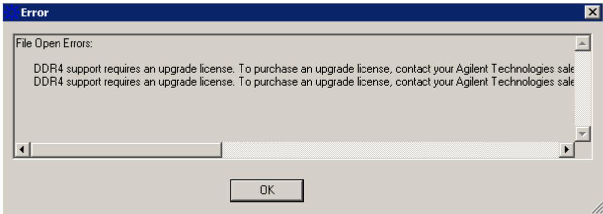
DDR4 configuration files require the B4621B upgrade license. Contact Agilent Technologies sales representative to purchase this upgrade license. Once you have installed this license, you can access all the available DDR files including DDR4 files.
