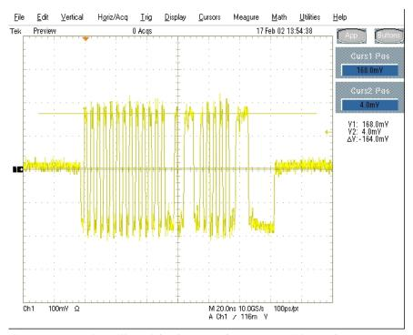
Figure 31: Measuring Differential Voltage Level – Zero to Positive Peak
