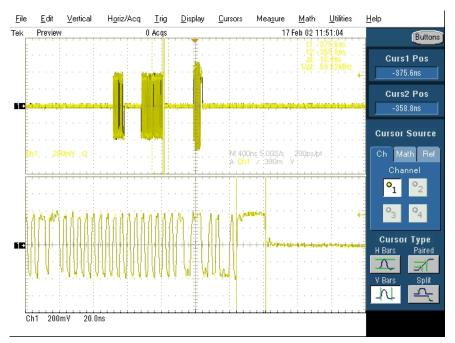
Figure 13: EOP in Device's Packet
