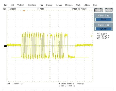
Figure 34: Measuring Differential Voltage Level - Zero to Negative Peak
