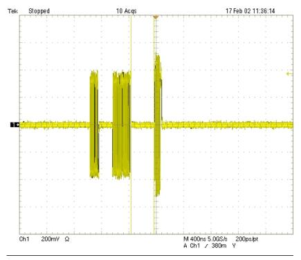
Figure 14: Device Inter-packet Gap
