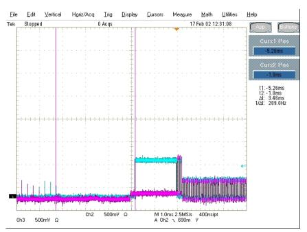
Figure 24: Device Chirp-K in Response to Reset from High-speed
