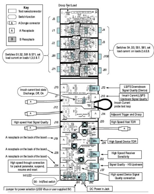
Figure 1: Tektronix TDSUSBF Test Fixture
