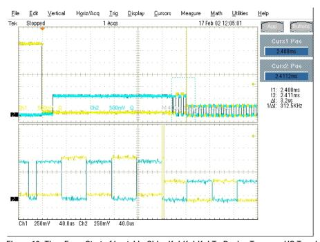
Figure 18: Time From Start of Last J in Chirp K-J-K-J To Device Turns on HS Termination
