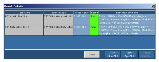
Figure 208: Result Details for Jitter Tolerance
