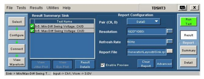
Figure 196: Result for Min/Max-Diff Swing Tolerance
