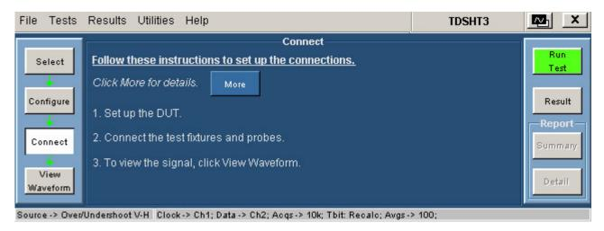
Figure 137: Connect pane for Over/Undershoot V-H
