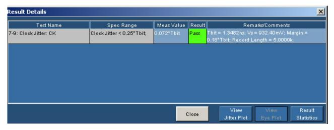
Figure 133: Result Details for Clock Jitter
