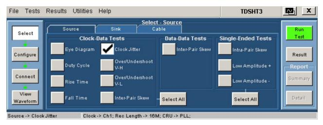
Figure 127: Select Source with Clock Jitter test selected
