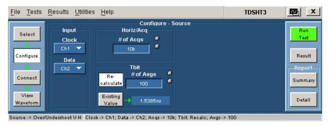
Figure 136: Configure Source for Over/Undershoot V-H
