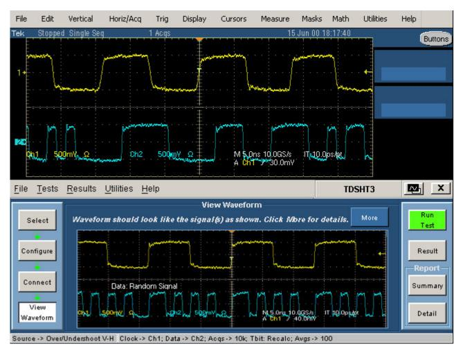
Figure 138: Waveform of Over/Undershoot V-H
