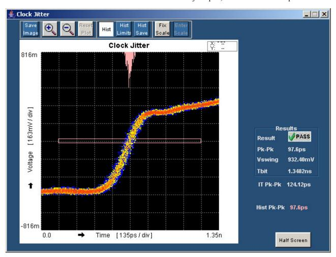
Figure 131: Clock Jitter plot
