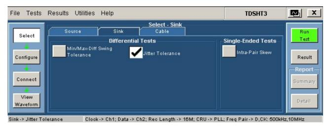
Figure 199: Select Sink with Jitter Tolerance test selected
