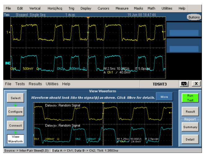
Figure 167: Waveform of Inter-Pair Skew (Data-Data)
