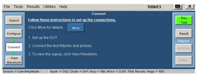
**8.** To connect the DUT, click **Tests** > **Connect**.
