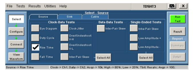
Figure 111: Select Source with Rise Time test selected
