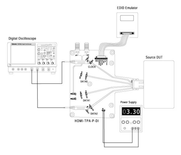
Figure 59: Connections for Source Fall Time
