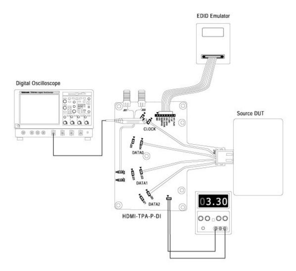
Figure 67: Connections for Source Intra-Pair Skew test (with Re-calculate Tbit option selected)
