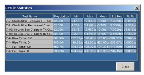
Figure 163: Result Details for Source Multiple Tests
