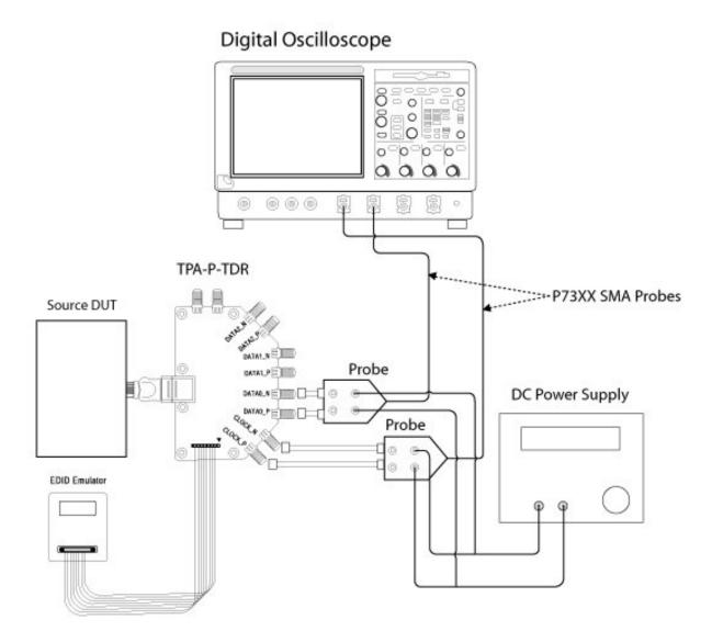
Figure 61: Connections for Source Over/Undershoot V-H
