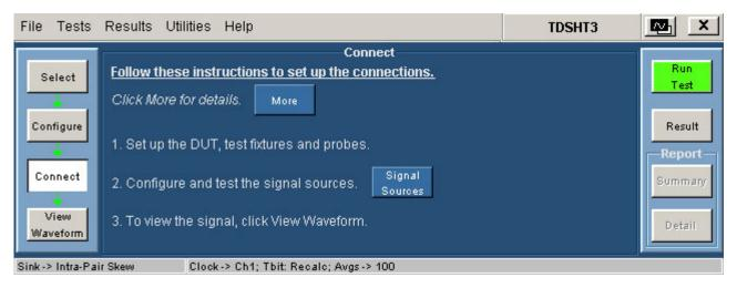
Figure 211: Connect pane for Sink Intra-Pair Skew
