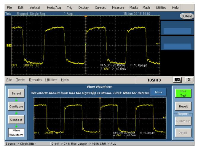
Figure 86: Waveform of Clock Jitter
