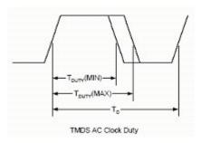
Figure 228: TMDS AC Clock waveform
