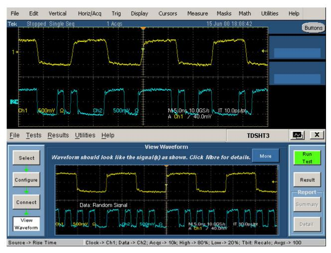
Figure 114: Waveform of Rise Time
