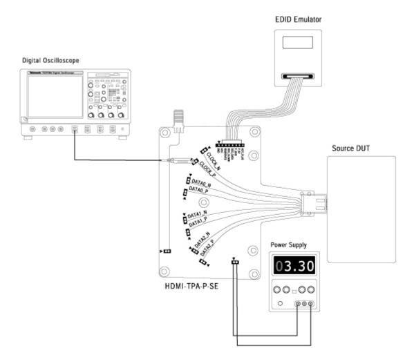
Figure 72: Connections for Low Amplitude - (with Existing Tbit option selected)
