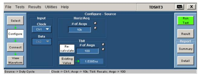
Figure 105: Configure Source for Duty Cycle
