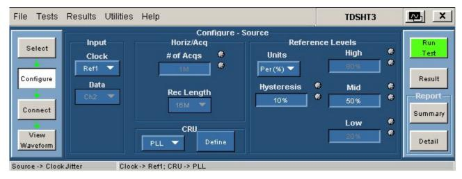
Figure 128: Configure Source for Clock Jitter
