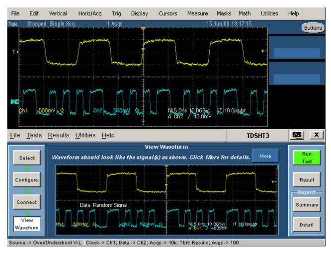
Figure 145: Waveform of Over/Undershoot V-L
