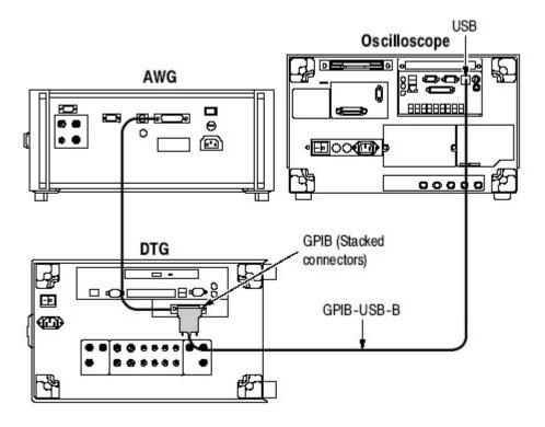
Figure 24: Connections for AWG/DTG (using GPIB-USB method)
