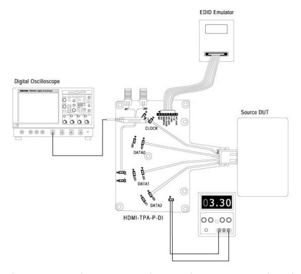
Figure 71: Connections for Low Amplitude - (with Re-calculate Tbit option selected)
