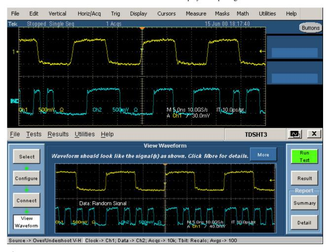
Figure 87: Waveform of Over/Undershoot V-H
