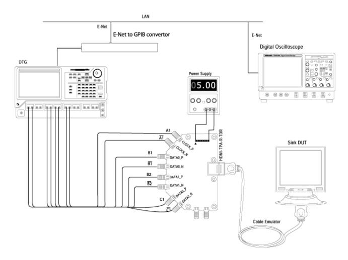
Figure 75: Connections for Min/Max-Diff Swing Tolerance (to find the maximum swing voltage of the Sink DUT)
