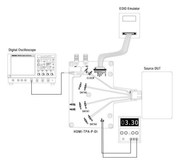
Figure 69: Connections for Low Amplitude + (with Re-calculate Tbit option selected)
