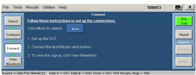
7. To connect the DUT, click **Tests** > **Connect**.
