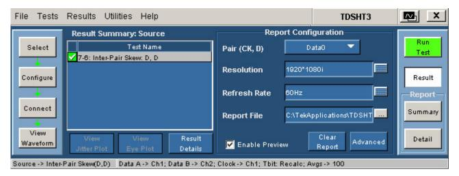
Figure 168: Result for Inter-Pair Skew (Data-Data)
