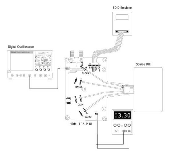
Figure 60: Connections for Source Clock Jitter
