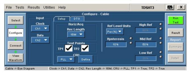
Figure 218: Configure Cable for Eye Diagram
