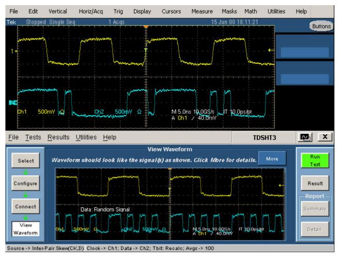
Figure 152: Waveform of Inter-pair Skew (Clock-Data)
