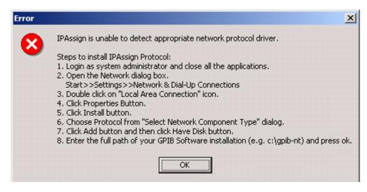
Figure 31: IP Assign Address message box
