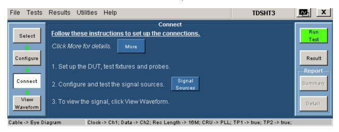
Figure 219: Connect pane for Cable Eye Diagram
