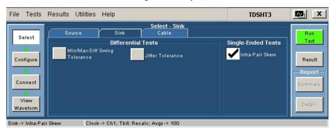
Figure 209: Select Sink with Intra-Pair Skew test selected
