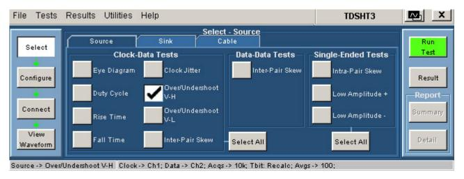
Figure 135: Select Source with Over/Undershoot V-H test selected
