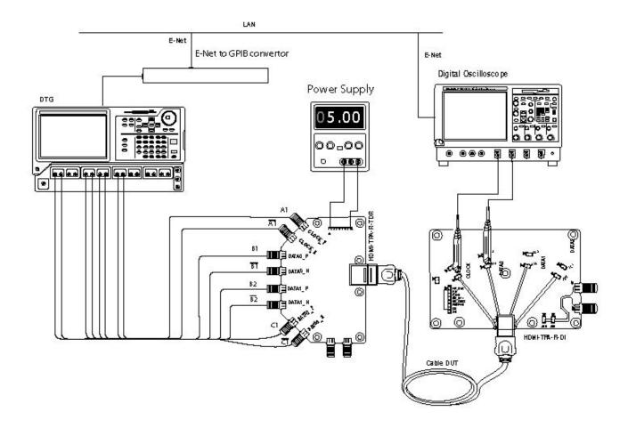
Figure 81: Connections for Cable Eye Diagram (Setup diagram for TP2)
