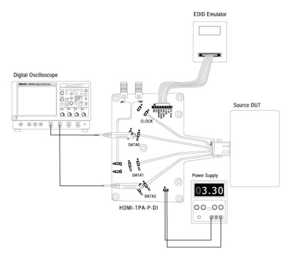
Figure 66: Connections for Source Inter-Pair Skew of Data-Data tests (with Existing Tbit option selected)
