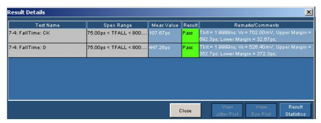
Figure 125: Result Details for Fall Time
