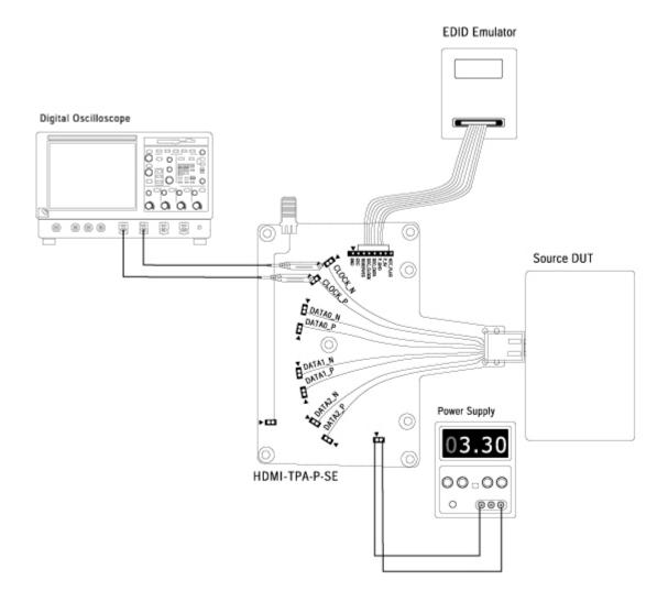
Figure 68: Connections for Source Intra-Pair Skew test (with Existing Tbit option selected)
