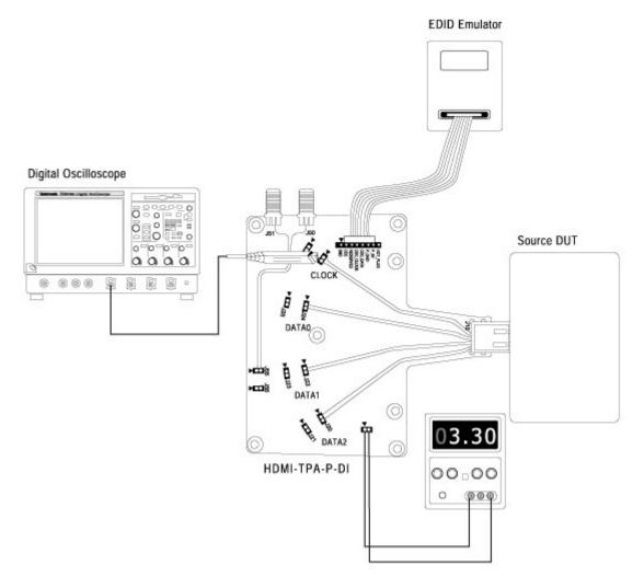
Figure 45: Connections to calculate Tbit
