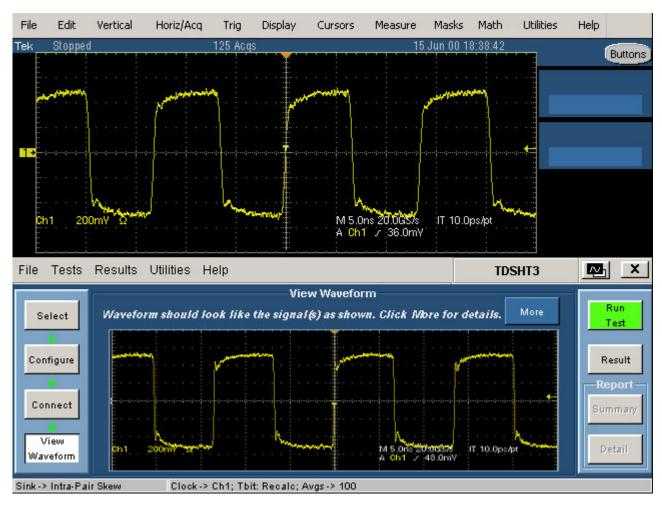
Figure 95: Waveform of Sink Intra-Pair Skew
