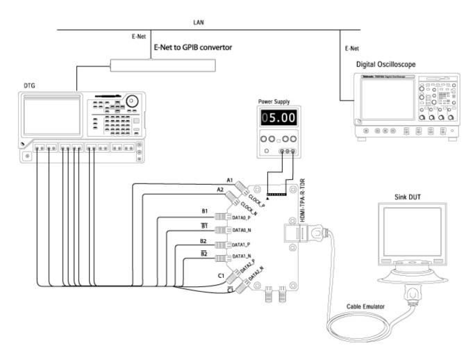
Figure 79: Connections for Sink Intra-Pair Skew (to find intra-pair skew of the Sink DUT)
