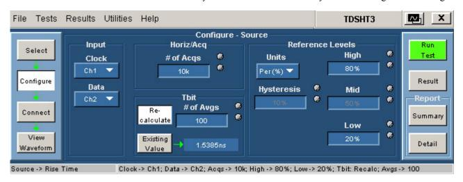
Figure 112: Configure Source for Rise Time
