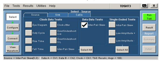
Figure 164: Select Source with Inter-Pair Skew (Data-Data) test selected
