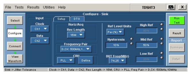
Figure 200: Configure Sink for Jitter Tolerance
