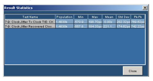
Figure 134: Result Statistics for Clock Jitter
