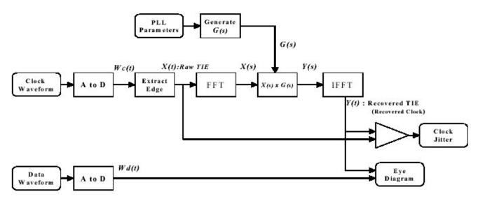
Figure 227: Proposed diagram of PLL design for CRU implementation
