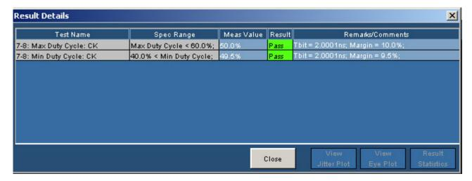
Figure 110: Result Details for Duty Cycle
