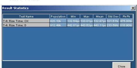
**13.** In the **Result Details** dialog box, click **Result Statistics** to display statistics based on the tests.
