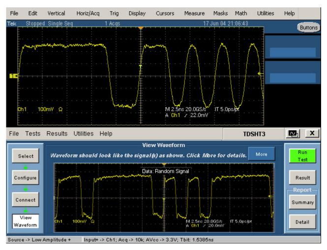
Figure 181: Waveform of Source - Low Amplitude + test
