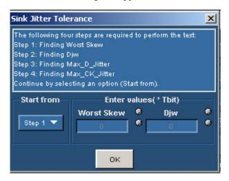
Figure 203: Sink Jitter Tolerance
