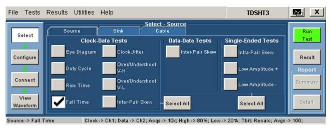
Figure 119: Select Source with Fall Time test selected
