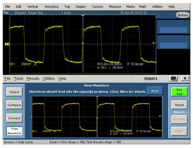
Figure 107: Waveform of Duty Cycle
