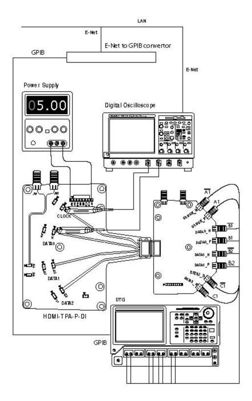
Figure 80: Connections for Cable Eye Diagram (Setup diagram for TP1)
