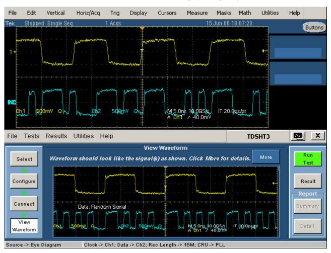
Figure 82: Waveform of Source Eye Diagram
