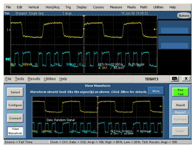
Figure 85: Waveform of Fall Time
