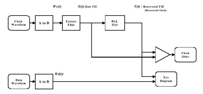
Figure 226: Conventional diagram of PLL design for CRU implementation
