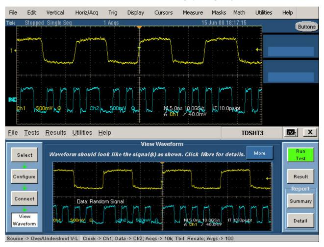
Figure 88: Waveform of Over/Undershoot V-L
