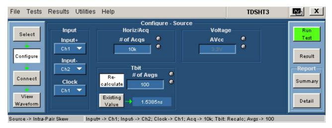
Figure 172: Configure Source for Intra-Pair Skew
