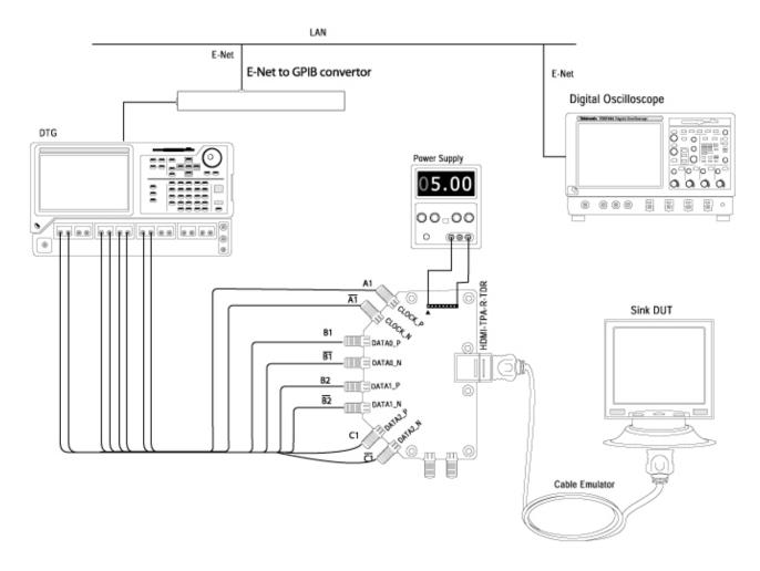
Figure 73: Connections for Min/Max-Diff Swing Tolerance (to find minimum swing voltage of the Sink DUT)
