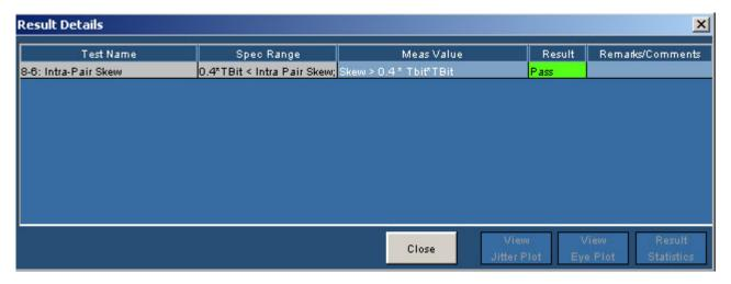
Figure 216: Result Details for Sink Intra-pair Skew
