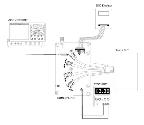
Figure 70: Connections for Low Amplitude + (with Existing Tbit option selected)
