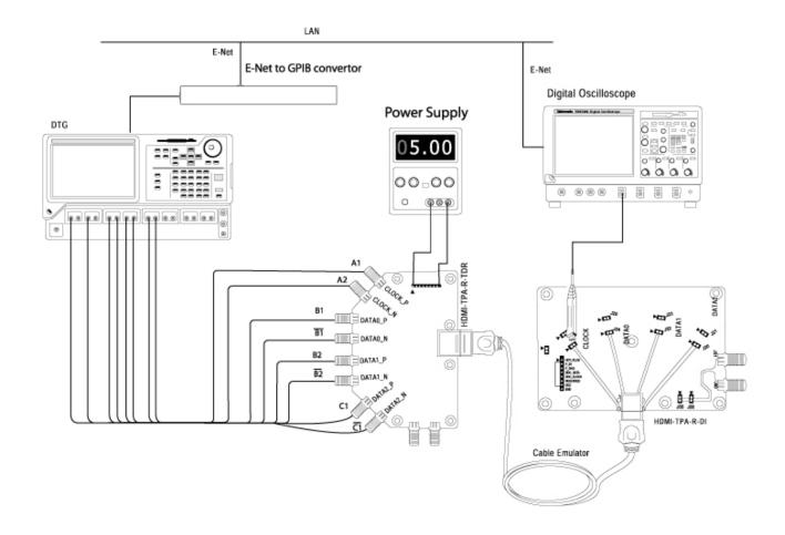
Figure 78: Connections for Sink Intra-Pair Skew (to measure Tbit)
