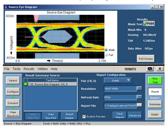
Figure 101: Waveform of Source Eye Diagram plot and Result
