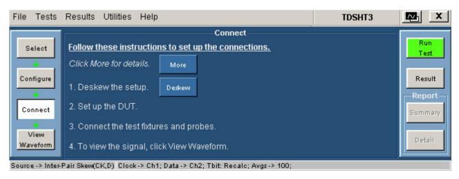
Figure 151: Connect pane for Inter-pair Skew (Clock-Data)
