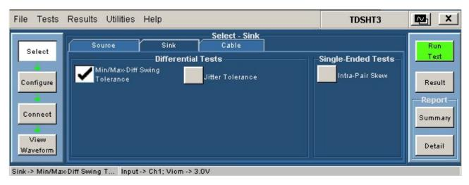
Figure 192: Select Sink with Min/Max-Diff Swing Tolerance test selected
