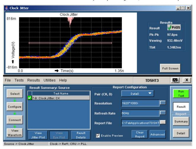
Figure 132: Source Clock Jitter plot and Result
