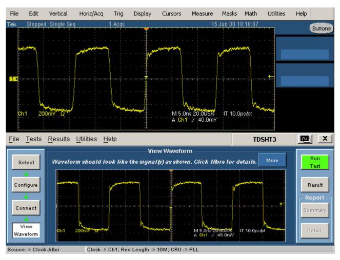
Figure 130: Waveform of Clock Jitter
