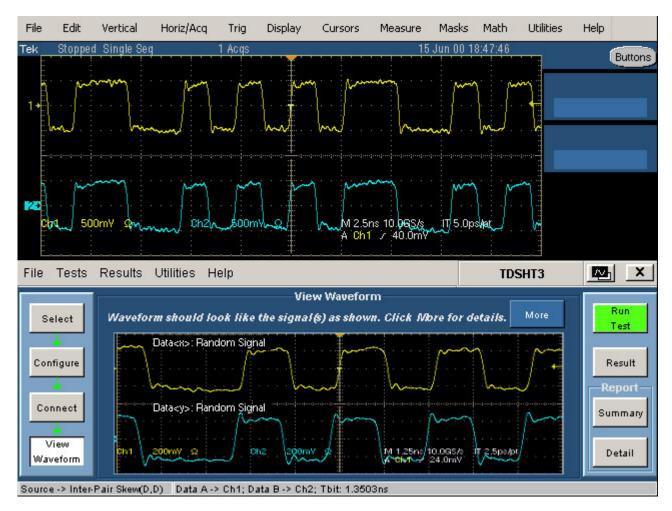
Figure 91: Waveform of Inter-Pair Skew (Data-Data)
