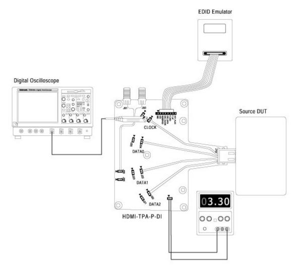
Figure 65: Connections for Inter-Pair Skew of Data-Data tests (with Re-calculate Tbit option selected)
