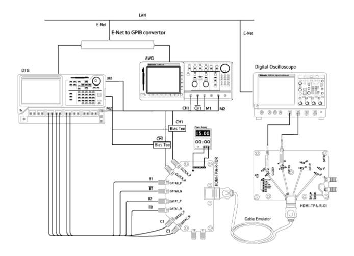
Figure 77: Connections for Jitter Tolerance (to measure the parameters)
