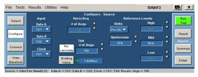
Figure 165: Configure Source for Inter-Pair Skew (Data-Data)
