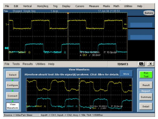
Figure 174: Waveform of Source Intra-Pair Skew
