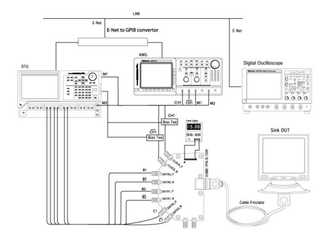
Figure 76: Connections for Jitter Tolerance (to find the device tolerance limit)
