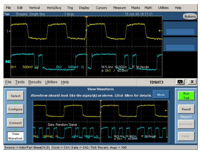
Figure 89: Waveform of Inter-Pair Skew (Clock-Data)
