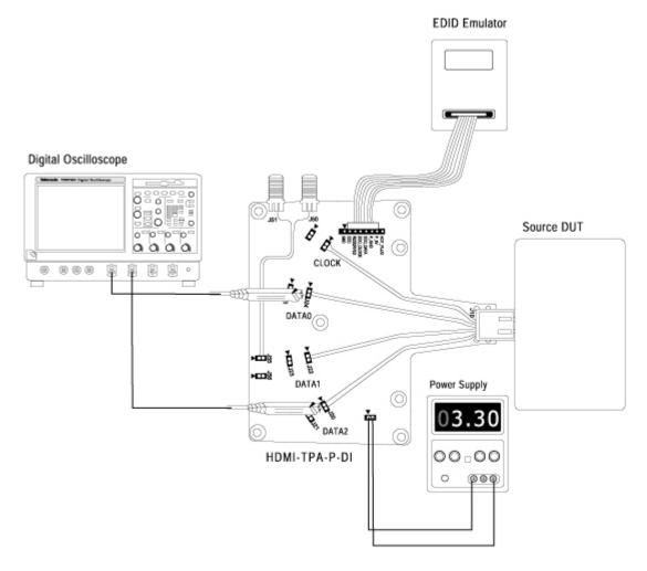
Figure 63: Connections for Inter-Pair Skew (Clock-Data)
