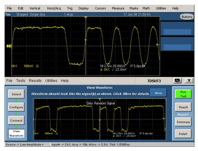
Figure 93: Waveform of Low Amplitude +
