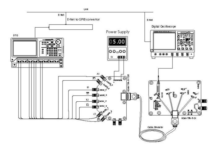
Figure 74: Connections for Min/Max-Diff Swing Tolerance (to measure the minimum differential swing voltage using an oscilloscope)
