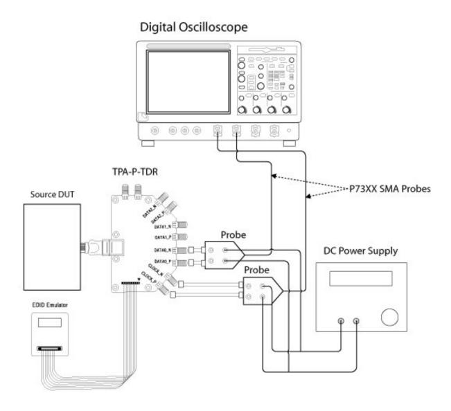
Figure 56: Connections for Source Eye Diagram
