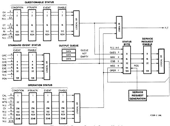
Figure 4-1. Power Supply Status Model
