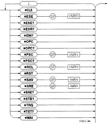
Figure 3-1. Common Commands Syntax Diagram
