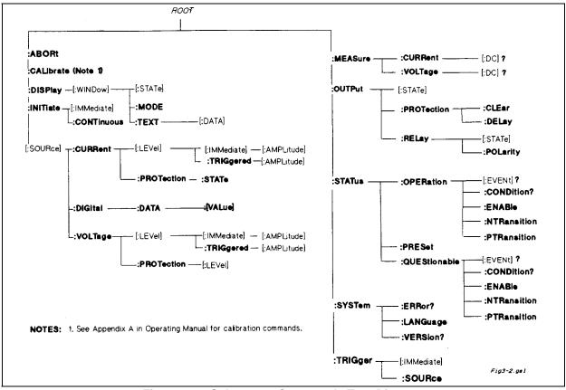
Figure 3-2. Subsystem Commands Tree Diagram
