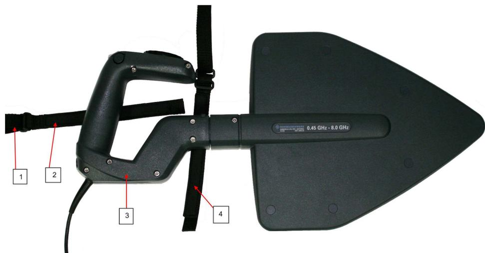
**Fig. 2-5: Attaching the belt, step 1.**
