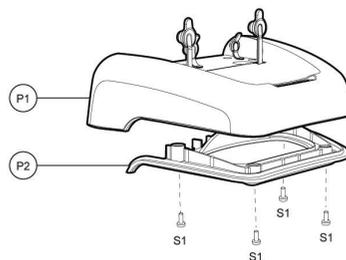
**Figure 3-13: Assembling the TOP HOLSTER**
