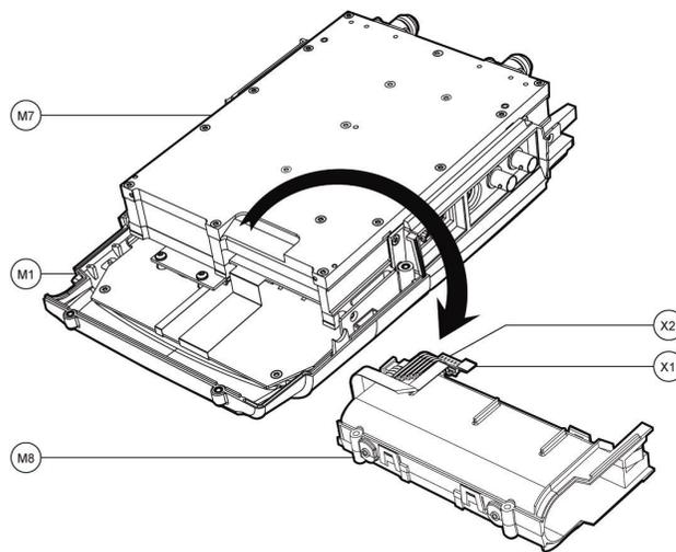
Figure 3-19: Remove BATTERY MODULE
