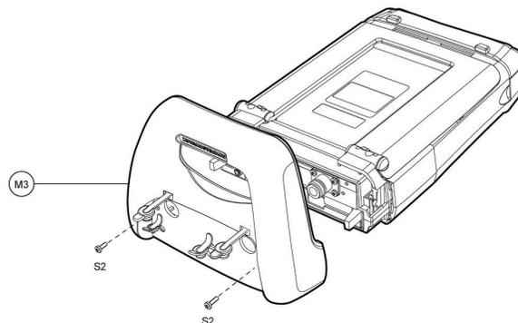
**Figure 3-14: Replacing the top holster**
