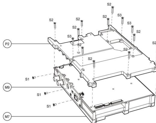
**Figure 3-35: Place the MAINBOARD SHIELDING ASSY**
