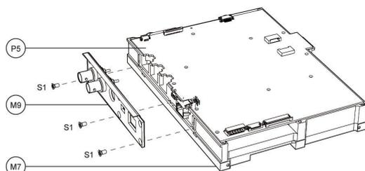
**Figure 3-37: Replace the CONNECTOR BRACKET**
