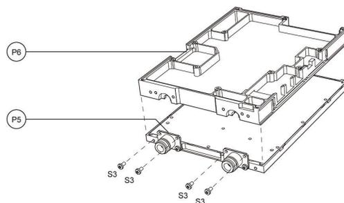
**Figure 3-42: Remove the COMBI SHIELD**
