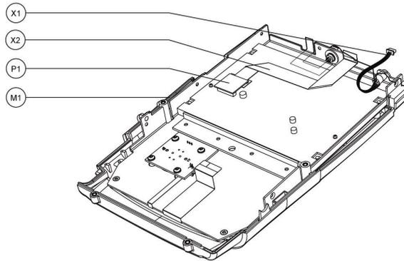
Figure 3-45: Replace AUDIO CABLE ASSY, LCD FLAT CABLE 30P, LCD SMD
