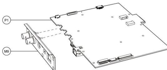
**Figure 3-33: Assemble the CONNECTOR BRACKET to the MAIN BOARD PCB**
