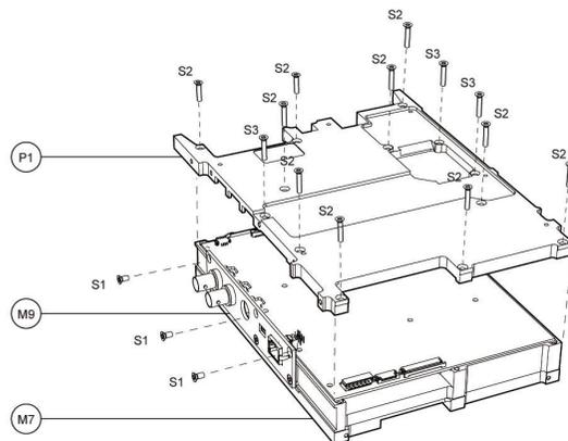
Figure 3-31: Remove MAINBOARD SHIELDING ASSY
