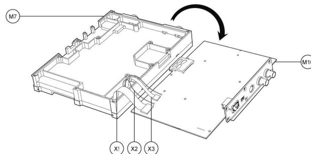
Figure 3-46: Replace MAINBOARD-RF FLAT CABLE 26P, MAINBOARD-RF CABLE 12P, COAX CABLE
