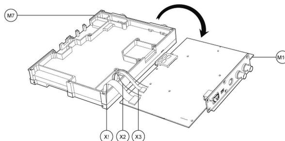
**Figure 3-39: Replace MAINBOARD-RF FLAT CABLE 26P, MAINBOARD-RF CABLE 12P, COAX CABLE**
