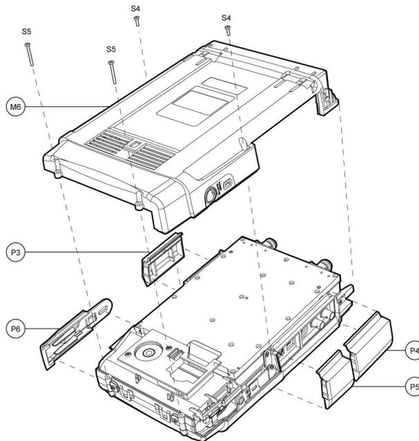
**Figure 3-5: Removing REAR CASE, CONNECTOR COVERS, and BATTERY DOOR**
