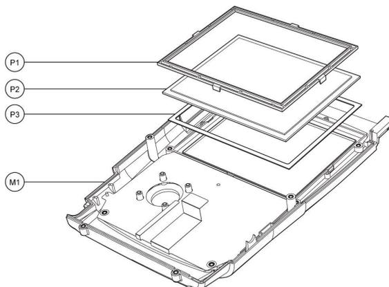
**Figure 3-30: Remove LENS SUPPORT FRAME and the LENS from the FRONT CASE**
