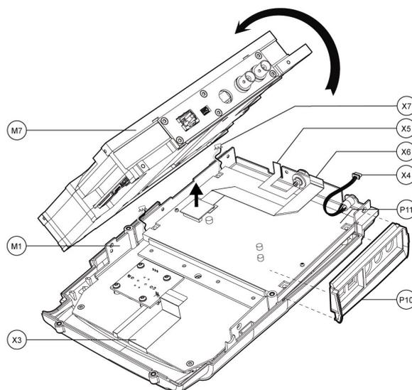
**Figure 3-23: Remove RF/IF MODULE to replace FRONT CASE MODULE**
