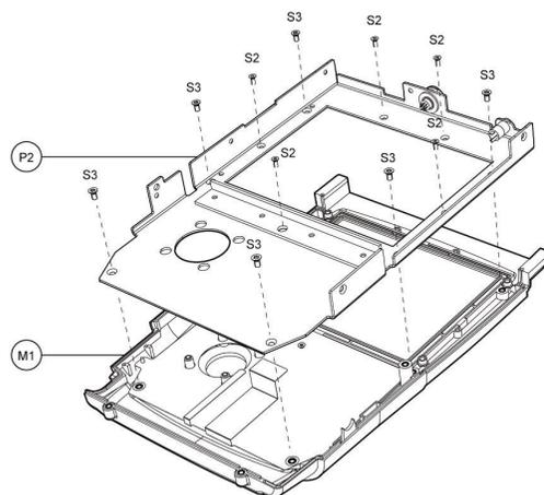
**Figure 3-28: Replace LCD SHIELDING**
