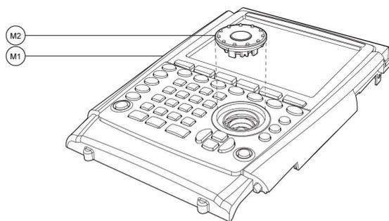
**Figure 3-25: Remove FRONT ROTARY out of the FRONT MODULE**
