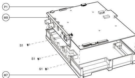
**Figure 3-38: Lift the MAINBOARD with CONNECTOR BRACKET**
