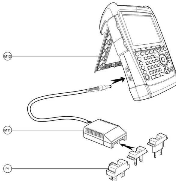
**Figure 3-51: Connect ADAPTER SET to POWER ADAPTER**
