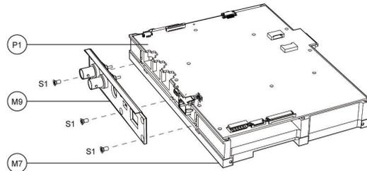
**Figure 3-34: Place the MAINBOARD and the CONNECTOR BRACKET in the RF/IF MODULE**
