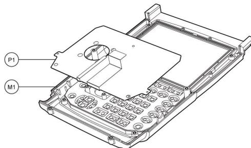
**Figure 3-29: Replace KEYPAD FOIL**
