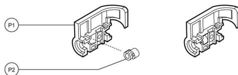
**Figure 3-15: Mounting the STANDUP HINGE SPRING into the STANDUP HINGE**
