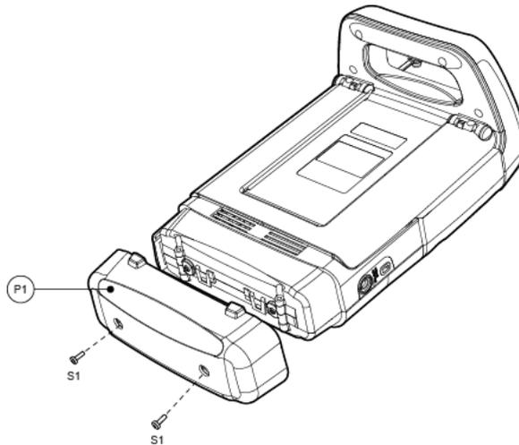
**Figure 3-12: Replacing the BOTTOM HOLSTER**
