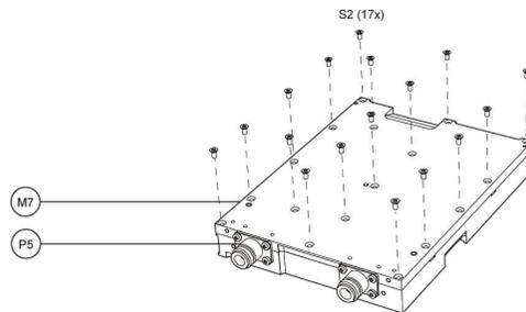
**Figure 3-41: Remove the screws at the rear of the RF/IF MODULE**
