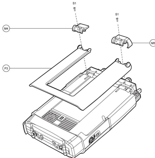
**Figure 3-16: Replacing the STAND-UP**
