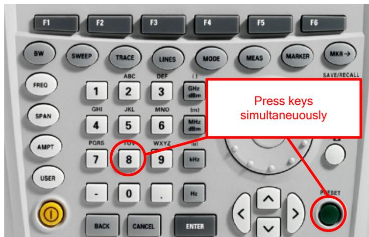
5. Keep PRESET and 8 pressed for at least 5 seconds after the startup screen has appeared on the screen
