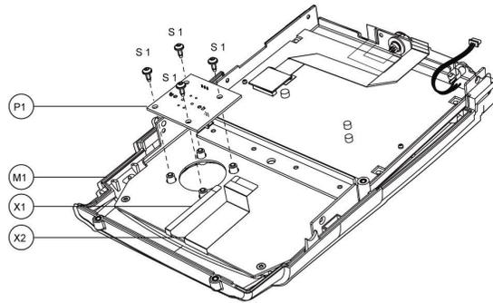
**Figure 3-26: Remove ROTARY PRINT from FRONT MODULE**
