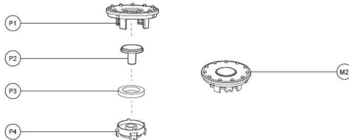
**Figure 3-10: Assemble the ROTARY ASSEMBLY**
