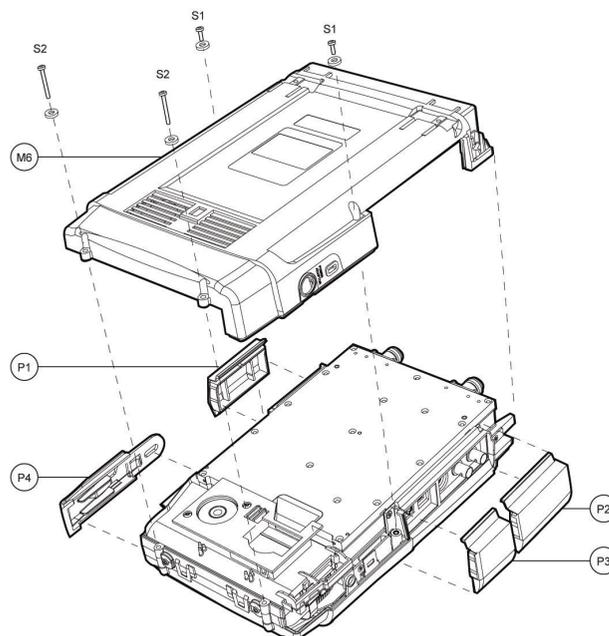
**Figure 3-17: Replacing the CONNECTOR COVER LEFT, RIGHT and BATTERY COVER**
