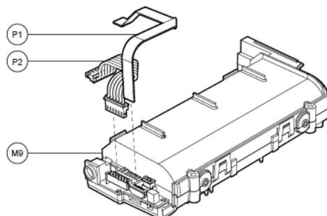
**Figure 3-44: Replace ADAPTION FLAT CABLE and ADAPTION CABLE 6P**
