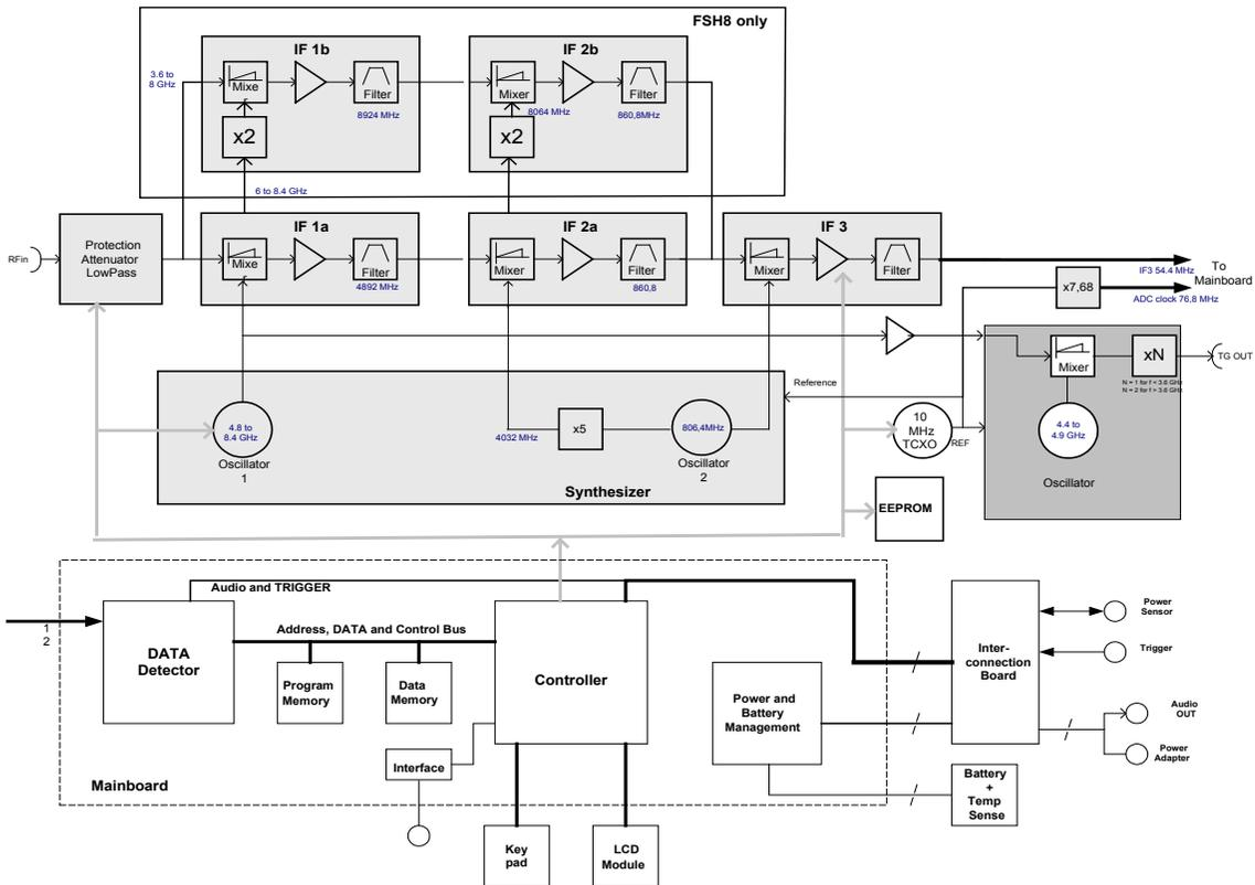
Figure 3-1: Block diagram of the R&S FSH
