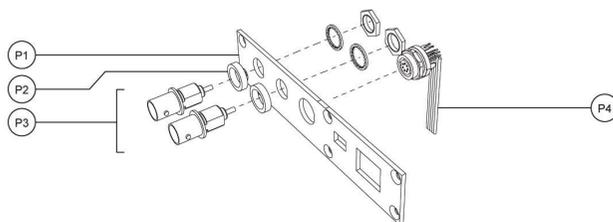
**Figure 3-36: Assemble the parts of the new CONNECTOR BRACKET**
