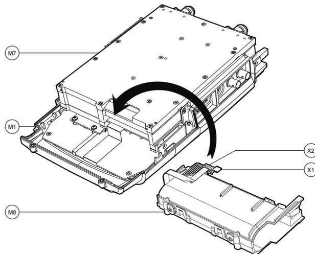
**Figure 3-21: Place BATTERY MODULE**
