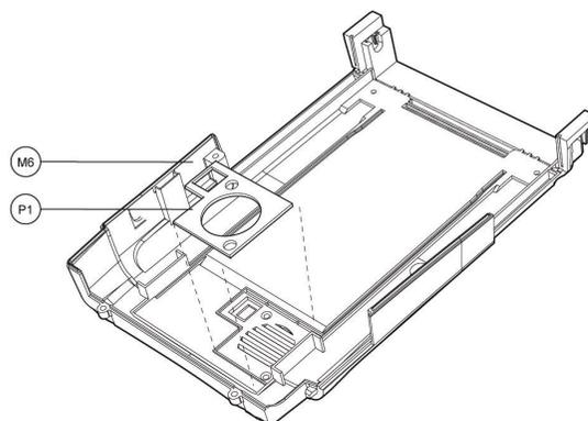
*Figure 3-18: Replace SPEAKER SEAL in REAR CASE*
