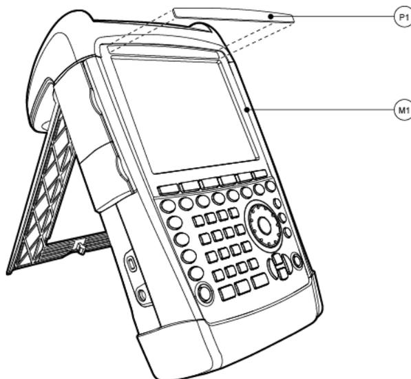
Figure 3-9: Replacing the Front decal sticker
