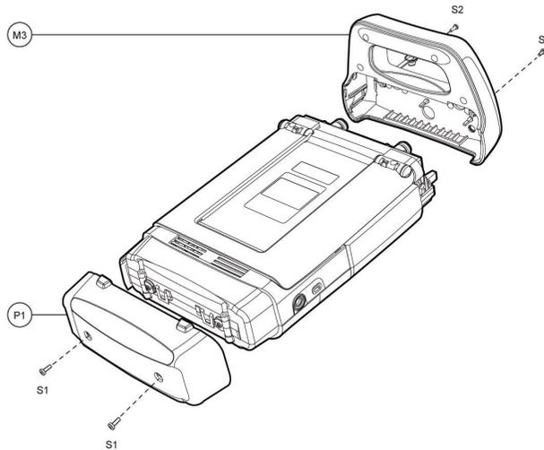
**Figure 3-3: Removing BOTTOM HOLSTER and TOP HOLSTER**
