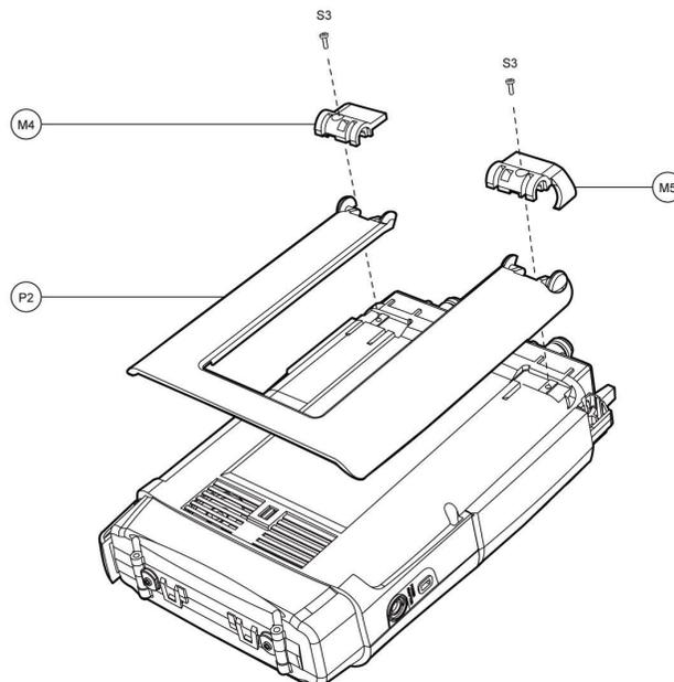
**Figure 3-4: Removing STANDUP**
