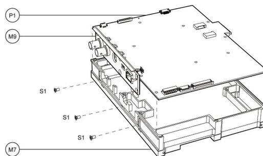
**Figure 3-32: Remove the MAINBOARD with CONNECTOR BRACKET**
