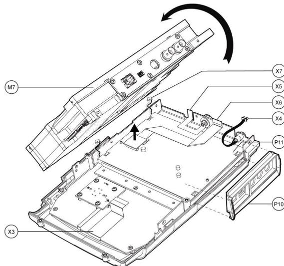
**Figure 3-8: Remove INTERNAL MODULE and SIDE PART RIGHT**
