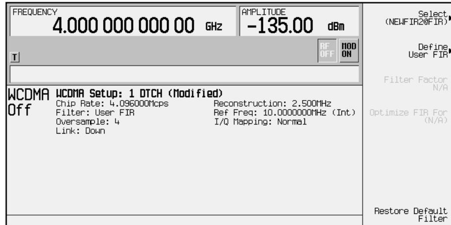
The filter you selected is NEWFIR2. You can see the name displayed below the **Select** softkey (at the top and right). In the Filter field, near the left of the display, **User FIR** is displayed to indicate that a user-defined FIR filter has been selected.
