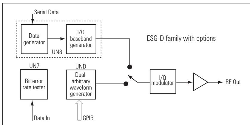
**Figure 1. Complementary digital baseband generation and bit-error-rate test in the Agilent ESG-D series**
