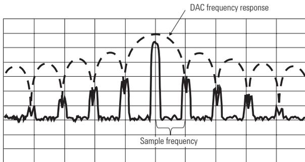
**Figure 22. Frequency response induced by sample-and-hold output of DACs**
