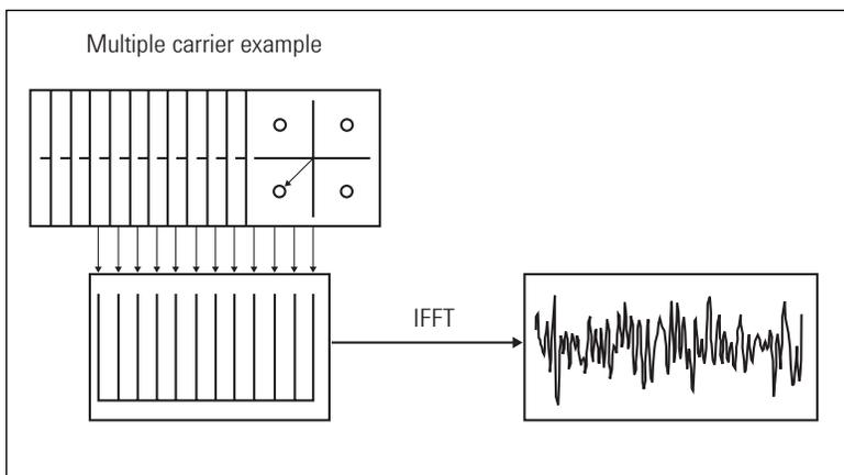
**Figure 25. Constructing an OFDM signal**
