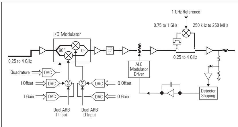
Figure 2. Block diagram of the Agilent ESG-D with dual arbitrary waveform generator
