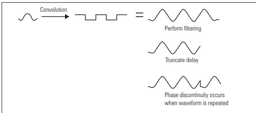
**Figure 16. Phase discontinuity generated by truncation after FIR filtering**
