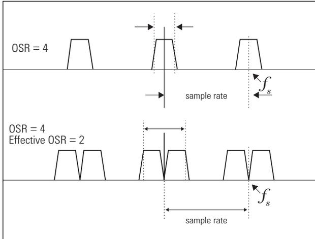
**Figure 20. Increased oversampling requirement for multi-carrier signals**
