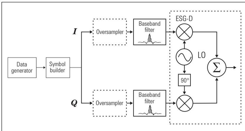
Figure 8. Block diagram of a basic digital transmitter
