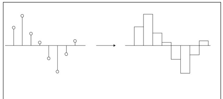
**Figure 21. Sample-and-hold DAC output compared to ideal digital synthesis**
