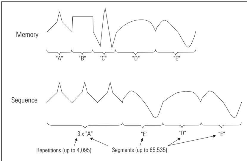
Figure 5. Using sequencing to conserve memory in the dual arbitrary waveform generator
