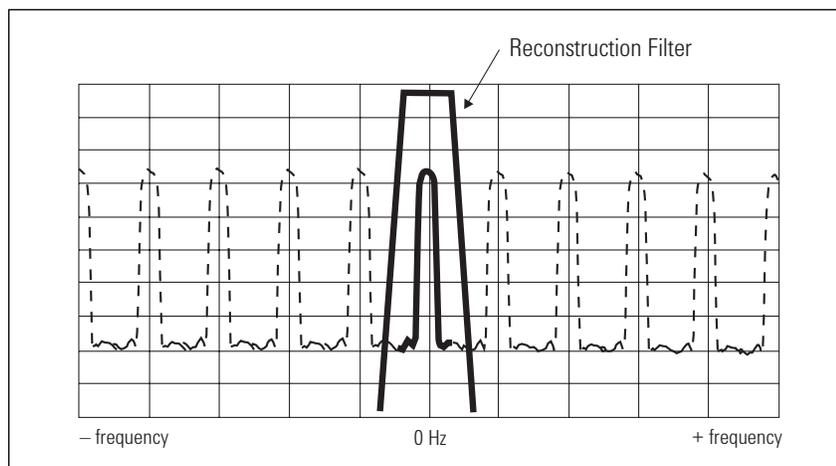
**Figure 7. The frequency-domain effect of time-domain sampling**
