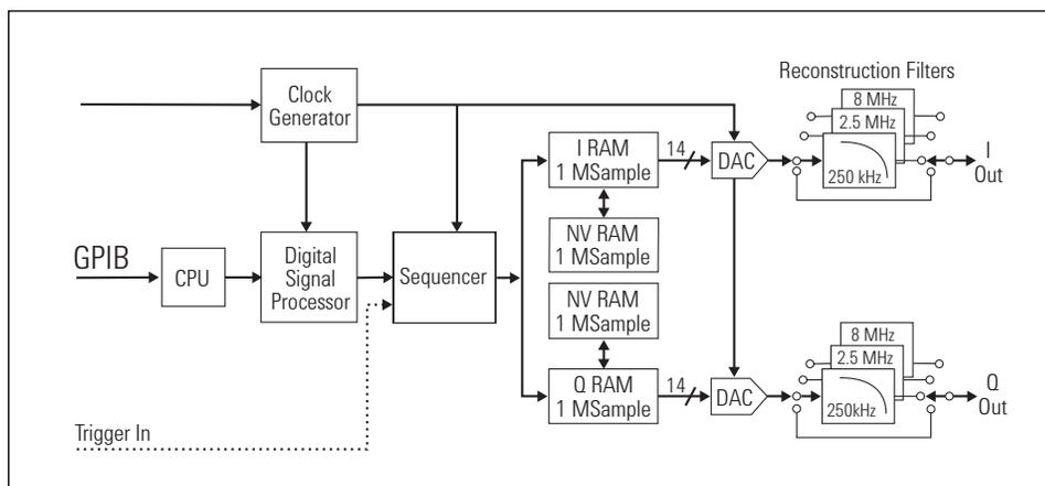
Figure 4. Agilent ESG series internal dual arbitrary waveform generator block diagram
