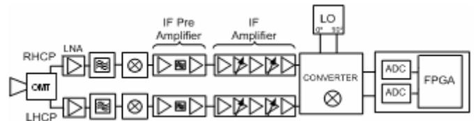
Fig. 2. Receiver overall block diagram.
