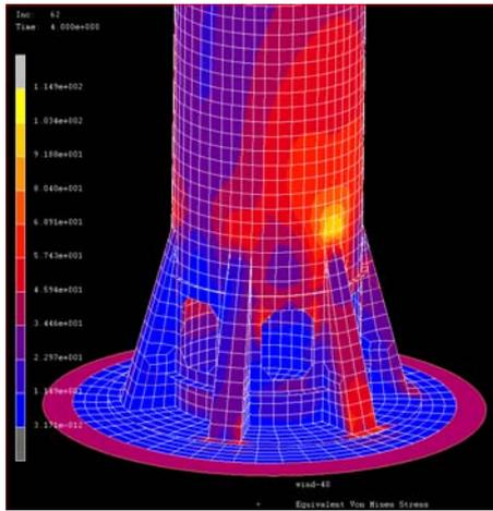
Fig. 5. Von Mises stress simulations for 40 Km/h wind speed load.
