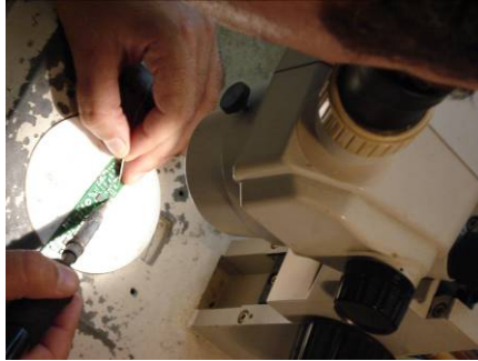
Figure 2 – Soldering the components
