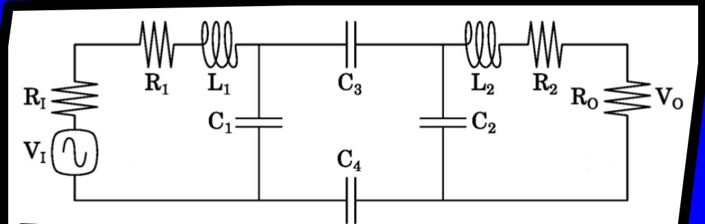
$$\frac{V_O}{V_I} = \frac{R_O Z_3}{Z_1 Z_2 \left( Z_3 \left[ jw(C_1 + C_2) + \frac{1}{Z_1} + \frac{1}{Z_2} \right] - w^2 C_1 C_2 + jw \left[ \frac{C_1 C_2}{Z_2 Z_1} \right] + \frac{1}{Z_1 Z_2} \right)}$$
