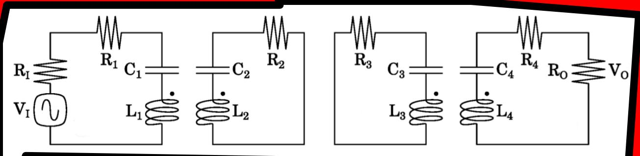
$$\frac{V_O}{V_I} = \frac{-jw^3 M_{12} M_{23} M_{34} R_O}{M_{12}^2 M_{34}^2 w^4 + Z_1 Z_2 Z_3 Z_4 + w^2 (M_{12}^2 Z_3 Z_4 + M_{23}^2 Z_1 Z_4 + M_{34}^2 Z_1 Z_2)}$$
