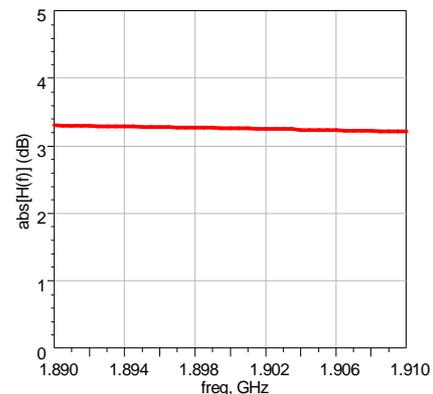
Fig. 5. Amplitude of the small signal gain variation with frequency of the nonlinear amplifier with memory considered.
