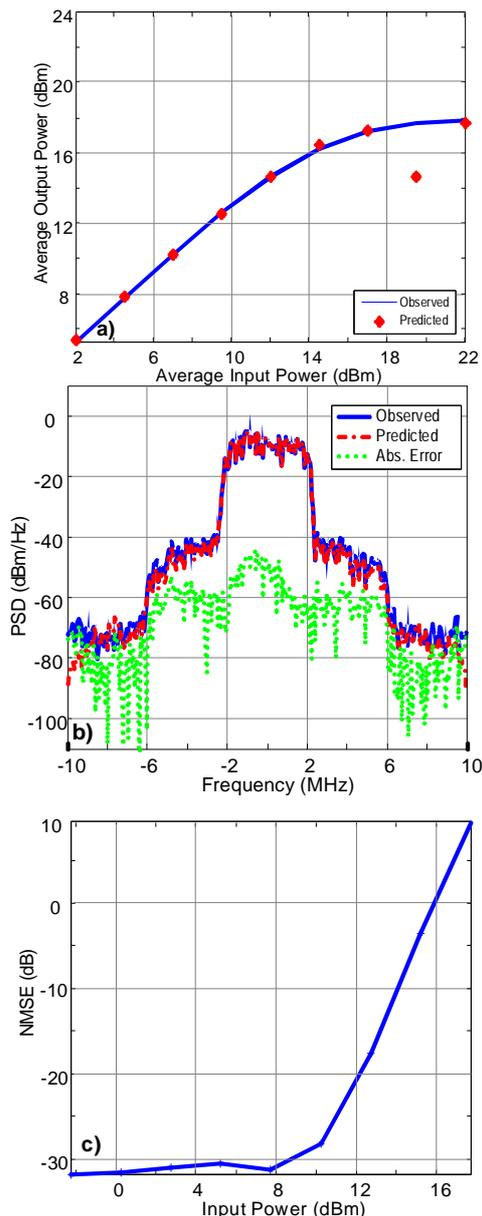
Fig. 8. Comparison of model and system responses. a) one tone PIN/POUT. b)WCMA spectra comparison. c) NMSE variation with average input power sweep for a WCDMA input stimuli.
