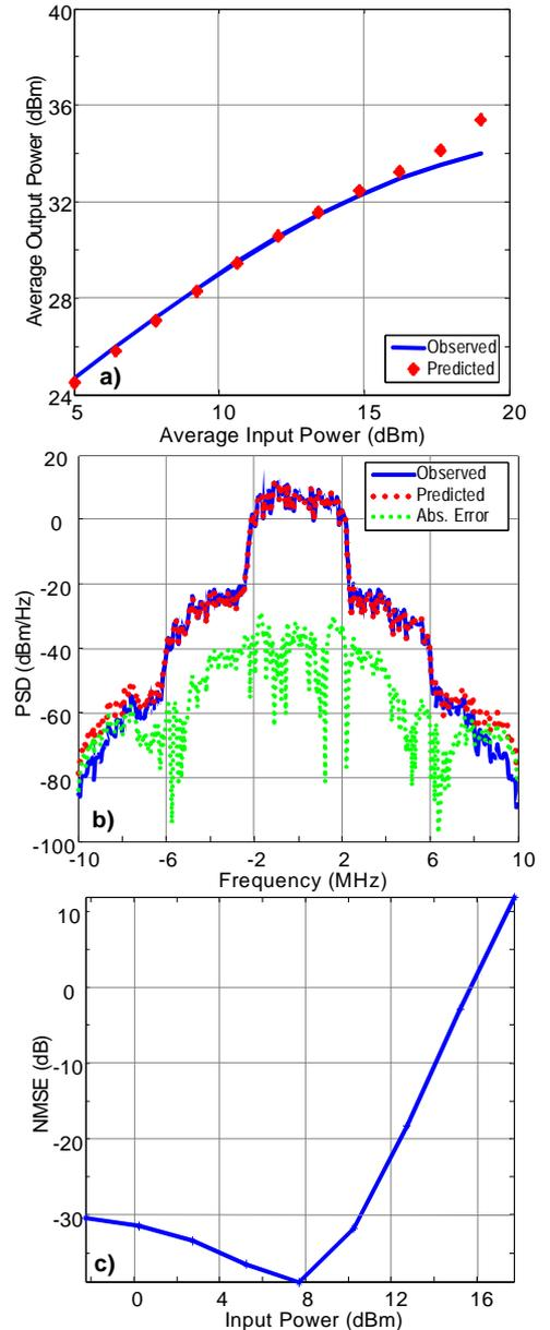
Fig. 7. Comparison of model and system responses. a) one tone  $P_{IN}/P_{OUT}$ . b) WCDMA spectra comparison. c) NMSE variation with average input power sweep for a WCDMA input stimuli.
