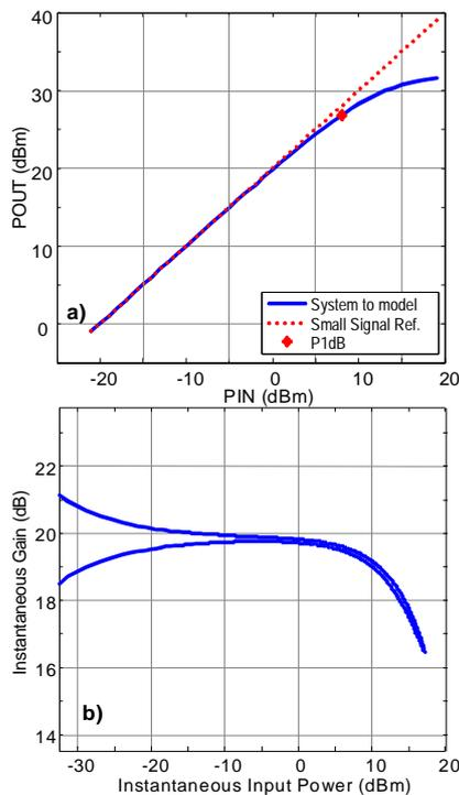
Fig. 3. a) One tone average  $P_{IN}/P_{OUT}$  of the system of Figure 2. b) Instantaneous two-tone Gain curve for the Wiener-Hammerstein configuration.
