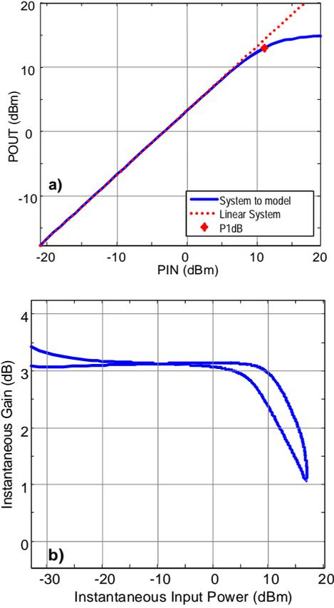
Fig. 6. a) One tone average  $P_{IN}/P_{OUT}$  of the system of Figure 2. b) Instantaneous two-tone Gain curve for the Wiener-Hammerstein configuration.
