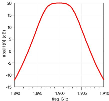
Fig. 2. Amplitude of the small signal gain variation with frequency of the considered Wiener-Hammerstein system.
