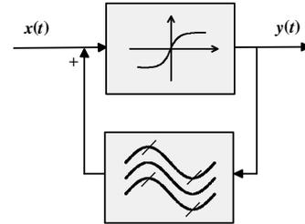
Fig. 4. Schematic representation of the Hammerstein model configuration.
