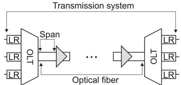
Fig. 1. Transmission system architecture composed by the optical fiber, the optical line terminal, the optical amplifier and the long reach transponders.
