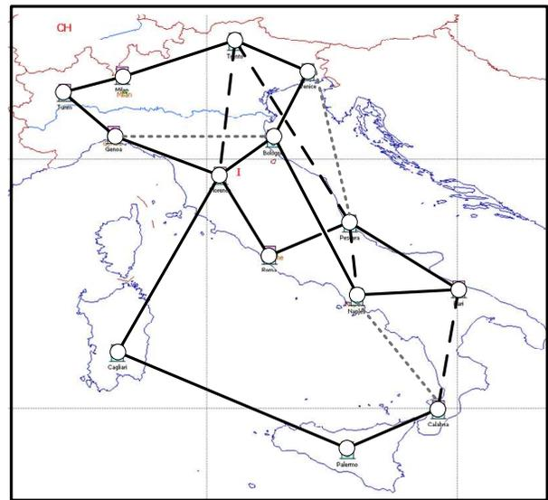
Fig. 5. Topologies in Italy obtained using the ILP model and the genetic algorithm. The dashed links differ in both solutions and the black links are common.
