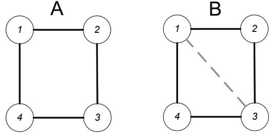
Fig. 2. Examples of solutions builded for the initial population. The ring topology displayed is common to all solutions. A random number of additional links are added in random locations, see the example B.
