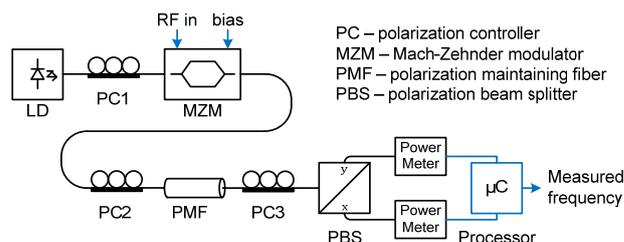
Fig. 1 Scheme of the proposed IFM system.
