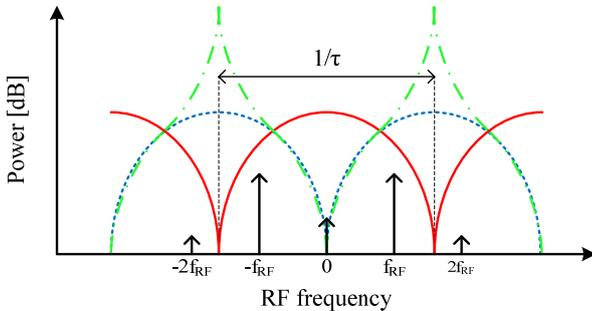
Fig. 2 Operation principle of the polarization-based interferometer. Constructive port (solid line), destructive port (dashed line) and ACF (dashed-dotted line).
