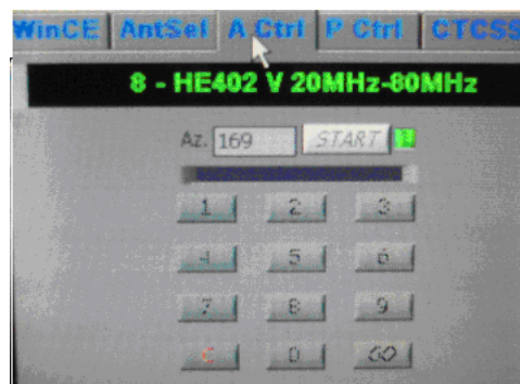
Fig. 7 Antenna azimuth control tab of the embedded software for touch screen interface
