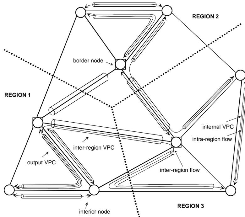
**Figure 1: 2-layer hierarchical virtual path layout**
