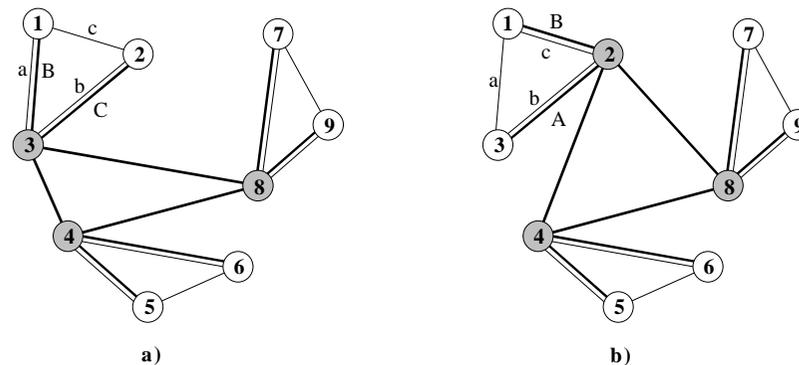
**Figure 3: Illustration on how to calculate intra-region VPC capacities**
