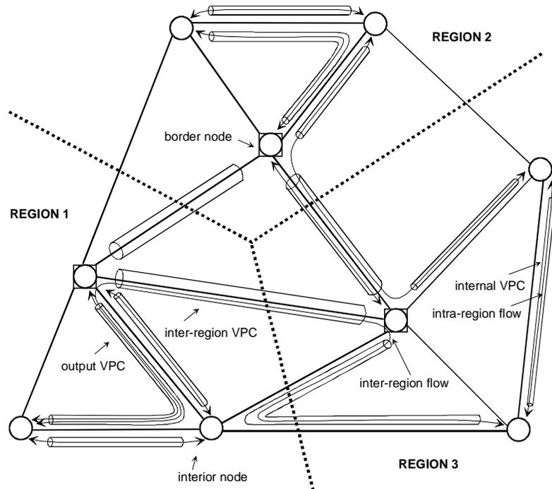
**Figure 1: 2-layer hierarchical virtual path layout**
