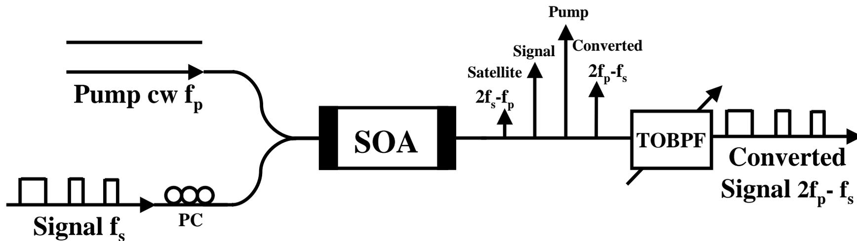
Carrier pulsation at the beating frequency causes index-gain grating which scatters the signal and the pump generating new frequencies.
