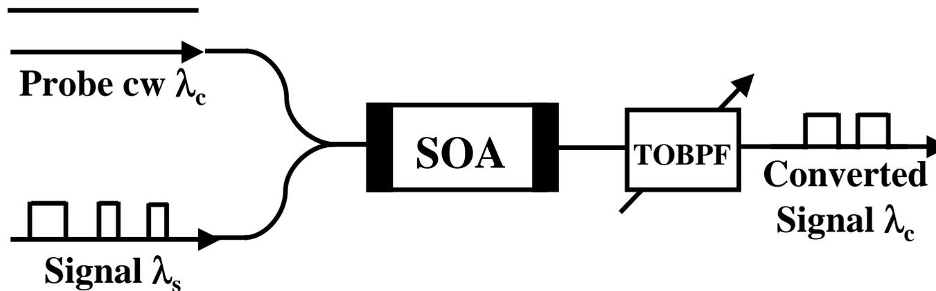
✚ Gain modulation due to the carrier depletion
