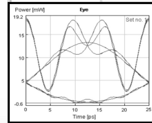
The pulses broadening is about  $\beta_2 / T_0$  per kilometer
