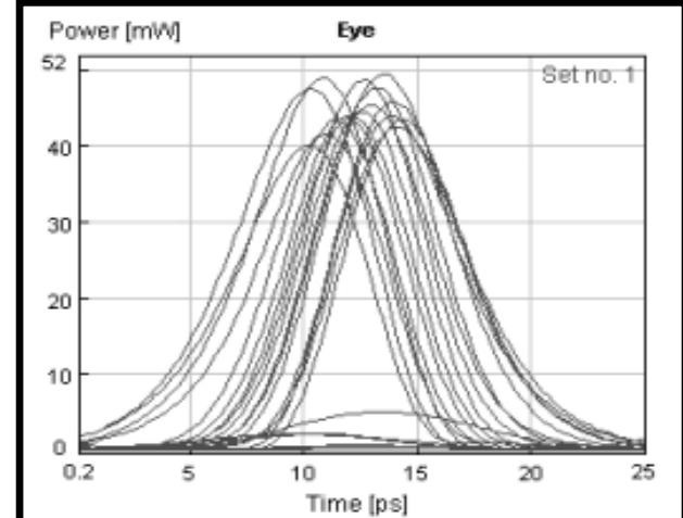
The SPM effect is not the main degradation effect
