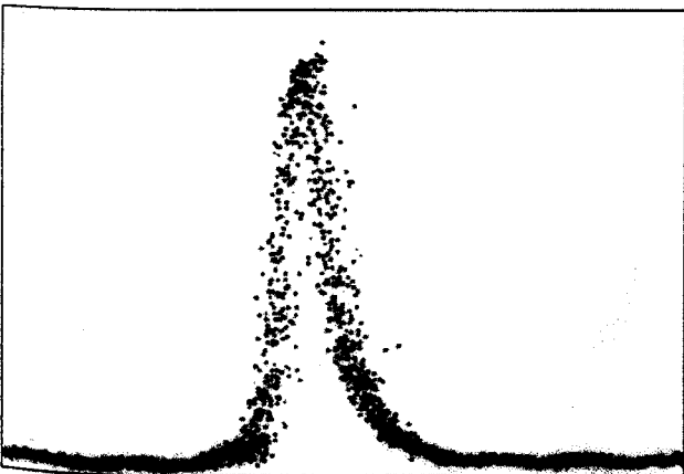
Fig. 11 - Photograph of the soliton pulse, obtained with a digital oscilloscope.
