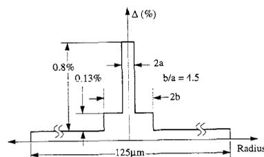
**TuO5 Fig. 1.** Refractive index profile of dual-shape-core dispersion shifted fiber.
