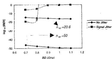
**TuO4 Fig. 3.** BER analytical estimates comparison with/without degradation due to signal jitter. The jitter statistics were estimated by simulation for  $n_{sp} = 20.6$  and  $n_{sp} = 50$ .
