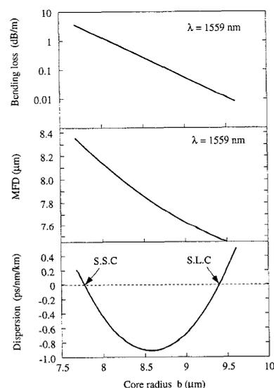
**TuO5 Fig. 2.** Bending loss, MFD and dispersion characteristics of dual-shape-core dispersion shifted fiber as a function of core diameter  $2b$ .
