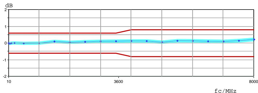
**8.3 RF attenuation 5 dB, AC coupled**
