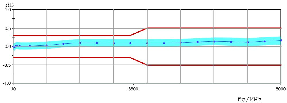
**8.6 RF attenuation 20 dB, AC coupled**
