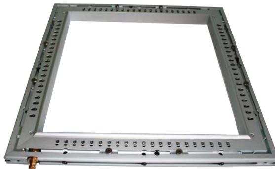
2. Carefully put the stencil onto the pins.
