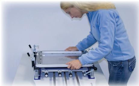
Roughly adjust the stencil frame over the PCB and test screen. Match cut shapes on the stencil with pads on the PCB. Lift up the frame.
