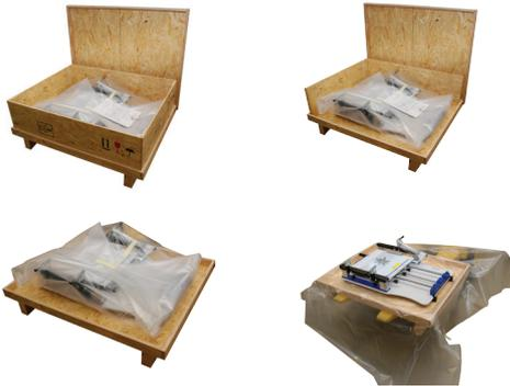
Remove wooden panel from each side. Open the plastic foil. Push the edge of the foil under the pallet.
