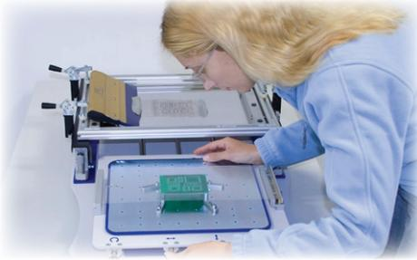
Align the PCB under the transparent test screen to accurately match orientation of the printed solder paste pattern with micro moving printing table in X, Y directions and rotation, using adjusting knobs located at the edge of the printing table.
