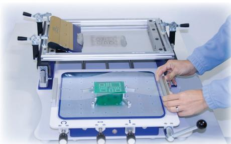
Remove the test print screen from the printing table.
