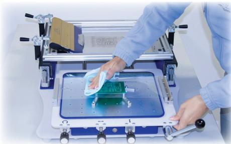
Clean the test print screen with soft a cloth, moistened in isopropyl alcohol.
