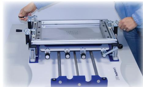
Fix the stencil frame with the toggle clamps.
