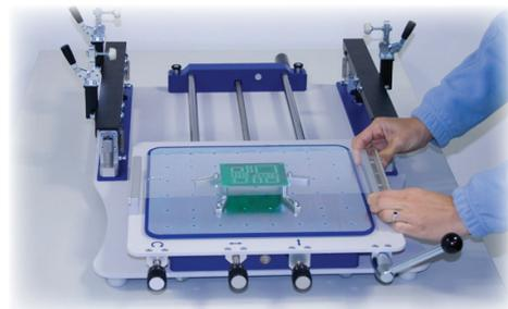
Place the test print screen over the PCB.
