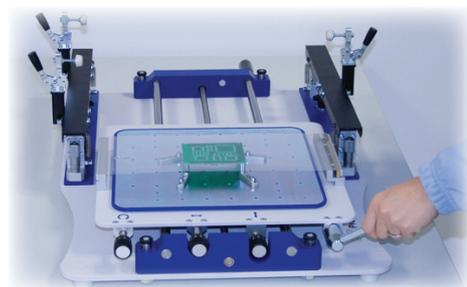
Push the printing table with the placed PCB and test screen to the print position, between support frames.
