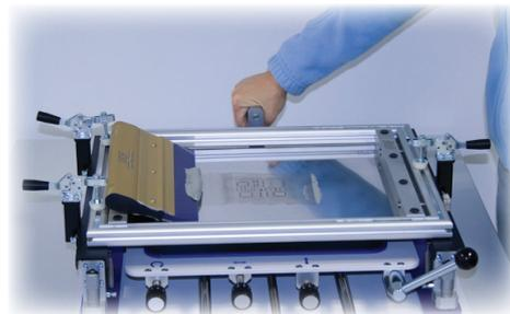
Separate the PCB and test screen from the framed stencil, using the elevating/release lever.
