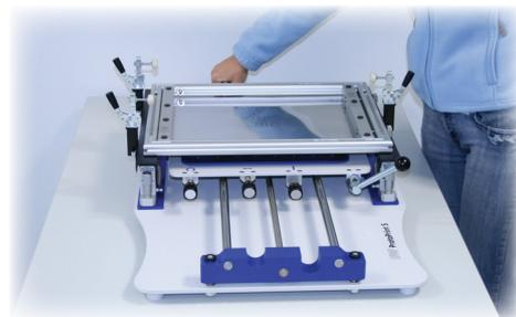
Use the elevating/release lever to bring the PCB and test screen into contact with the stencil.
