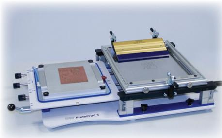
The vacuum table is equipped with special positioning pins, which ensures repeatability of the PCB position, when repeated printing is required.
