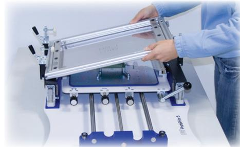
Mount the stencil frame with the attached stencil to the adjustable support frames.
