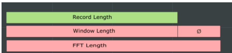
Fig. 5-20: FFT parameters for single FFT calculation
