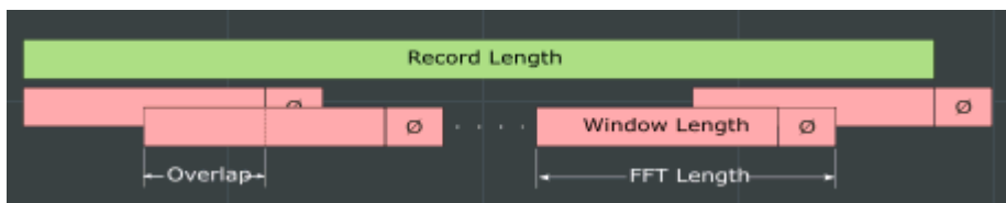
Fig. 5-21: FFT parameters for averaged FFT calculation
