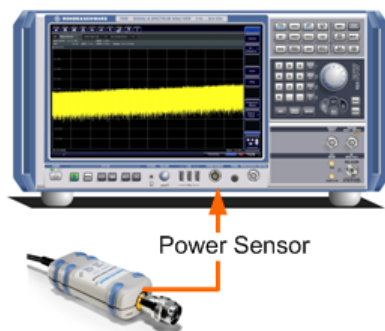
Fig. 6-3: Connecting a power sensor using the POWER SENSOR interface
