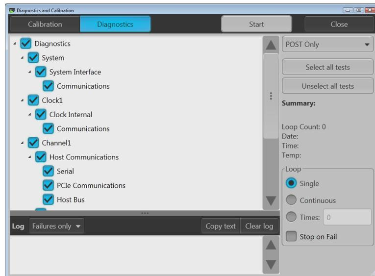
5. Select and deselect each test individually or use the **Select all tests** and **Unselect all tests** buttons.
