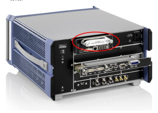
This removes all user data from the signal and spectrum analyzer. The signal and spectrum analyzer, **without** the removable solid-state drive, can now leave the secured area. Once the signal and spectrum analyzer is outside the secured area, installing a second **non-classified** removable solid-state drive (without any user data), allows the signal and spectrum analyzer to function properly for service or other needs.
