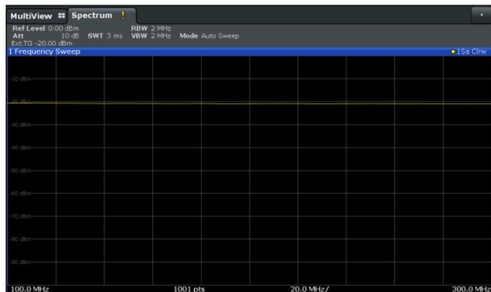
Fig. 6-7: Measurement results from generator, analyzer and connecting cables
