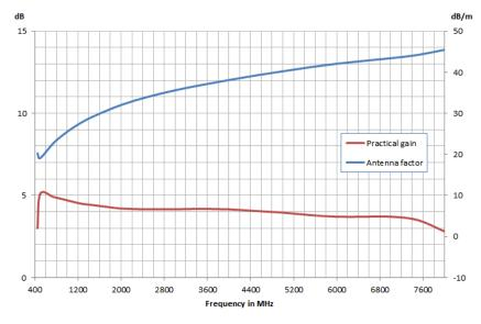
Fig. 5-2: R&S HL300 typical antenna factor and practical gain.
