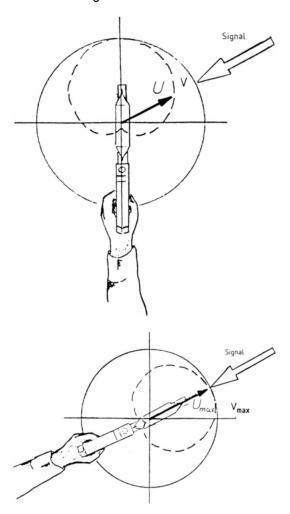
Fig. 3-5: Manual direction finding by locating the maximum.
