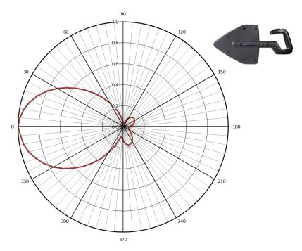
Fig. 5-3: R&S HL300 typical E-field pattern.
