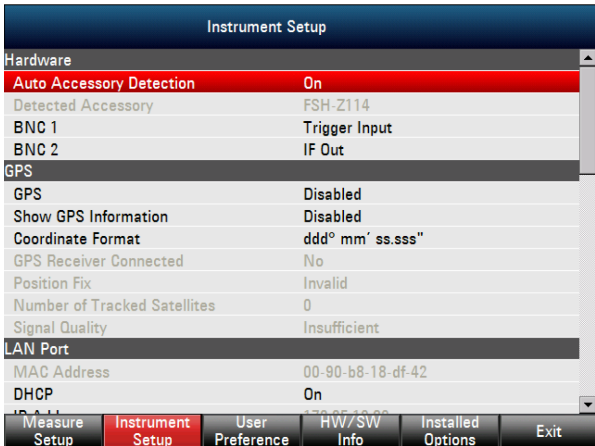
Fig. 3-2: Instrument setup for auto accessory detection
