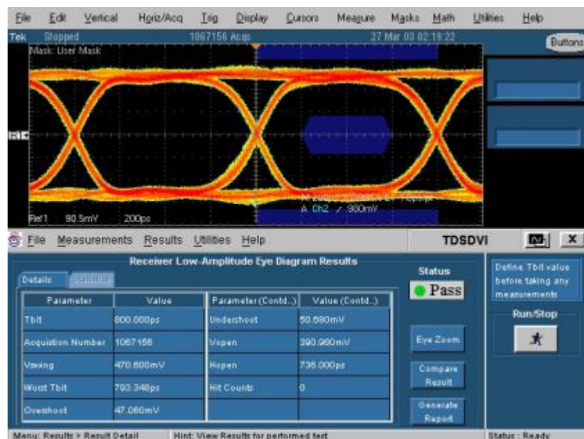
Figure 185: Low-Amplitude Eye diagram results
