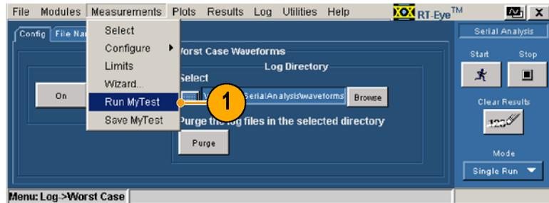
To run MyTest from the RT-Eye Welcome dialog box, which displays when you start the RT-Eye application, perform the following procedure:
