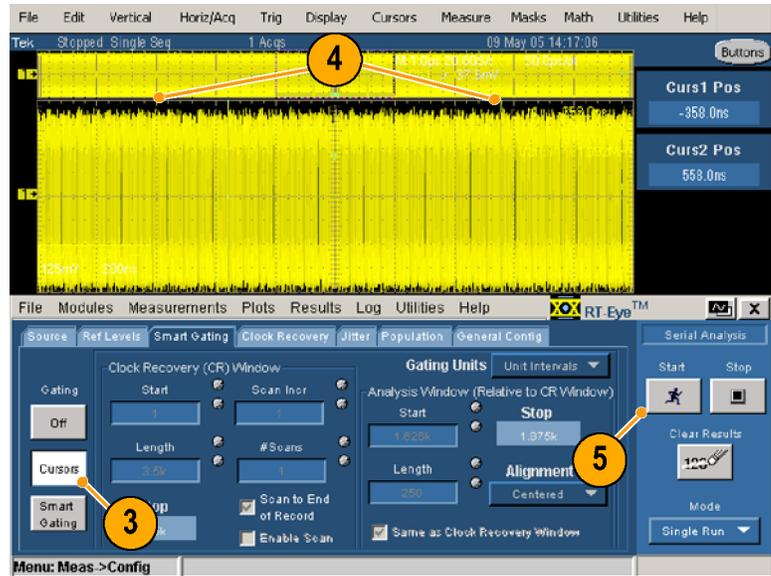
**Using Smart Gating to Set Up a Gated Region.** To set a gated region using smart gating, you must set up a Clock Recovery Window, and then define your gated region by setting up an Analysis Window within the Clock Recovery Window.
