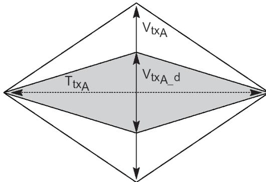
Figure 9: ExpressCard Module Transmitter compliance eye masks
