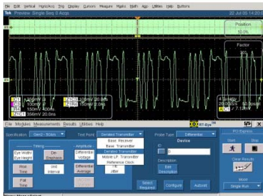
Figure 38: “De-rated Transmitter” DTP is now in the test point menu
