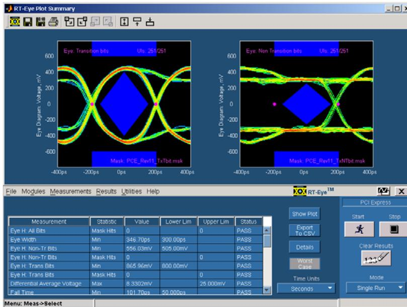
Figure 20: Result of a successful transmitter compliance test
