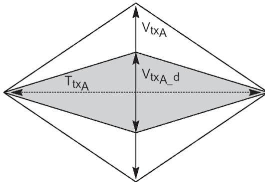
Figure 7: Cable (transmitter side) compliance eye masks
