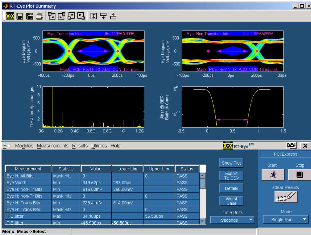
Figure 26: Successful add-in card compliance test
