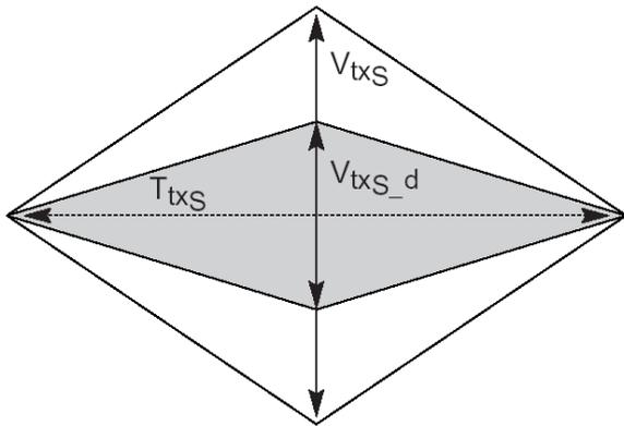
Figure 6: ExpressModule system board compliance eye masks
