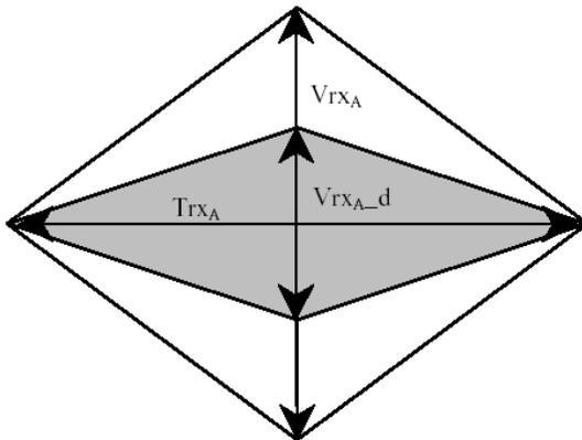
Figure 8: Cable (receiver side) compliance eye masks
