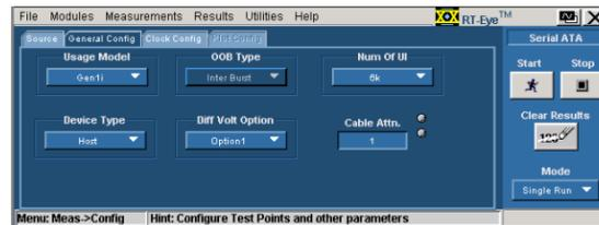
6. Push the “Running Man” button to start taking measurements. Follow the on-screen prompts to input different test patterns to complete the measurement. When the measurement is completed successfully, the application automatically displays the results. You can also view the results by selecting Results> Summary or Results> Details from the application menu bar.
